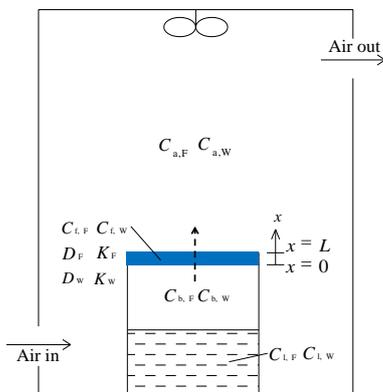
Figure 1: Schematic of emission model
