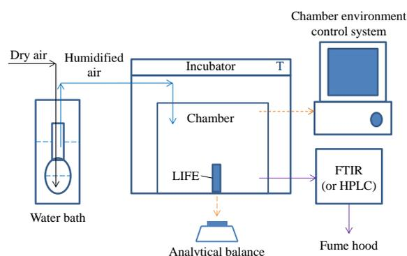
Figure 2: System for chamber test
