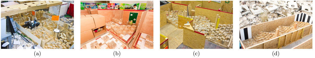
Figure 2: The evolution of the Stepfields standard test method apparatus through the course of the RoboCup competitions. (a) The initial Random Stepfield, as introduced in the 2005 competition. (b) The Symmetric Stepfields, the patterns for which were developed and refined during the 2008 competition. (c) The latest version of the Symmetric Stepfields, adapted for competition. (d) The final form of the Symmetric Stepfields in the test method.
