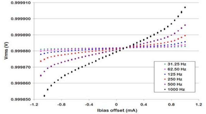
Fig. 2. PJVS rms voltage after full correction algorithm has been applied, including the final analysis that incorporates measurement bandwidth, rise time, and harmonic spectrum.
