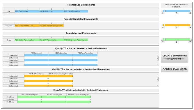
Figure 4. Example Interactive MRED Screen from Matlab Presenting the Available Environments and corresponding TTL – Environment relationship matrices
