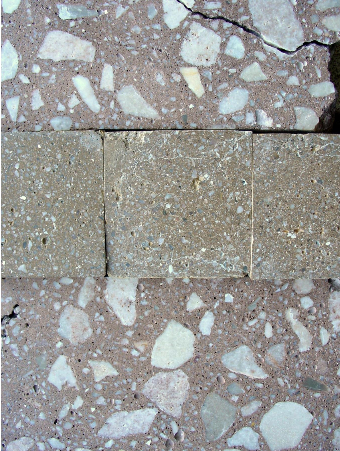
Figure 25. Comparison of the Valley of Fire cores #1 (upper) and #2 (lower) against 0.30 (left) 0.35 (center) and 0.40 (right) w/cm 50 mm cubes of lab mortar shows that the deck cores are redder in appearance, suggesting a lower w/cm ratio or possibly an increased dosage of pigment.
