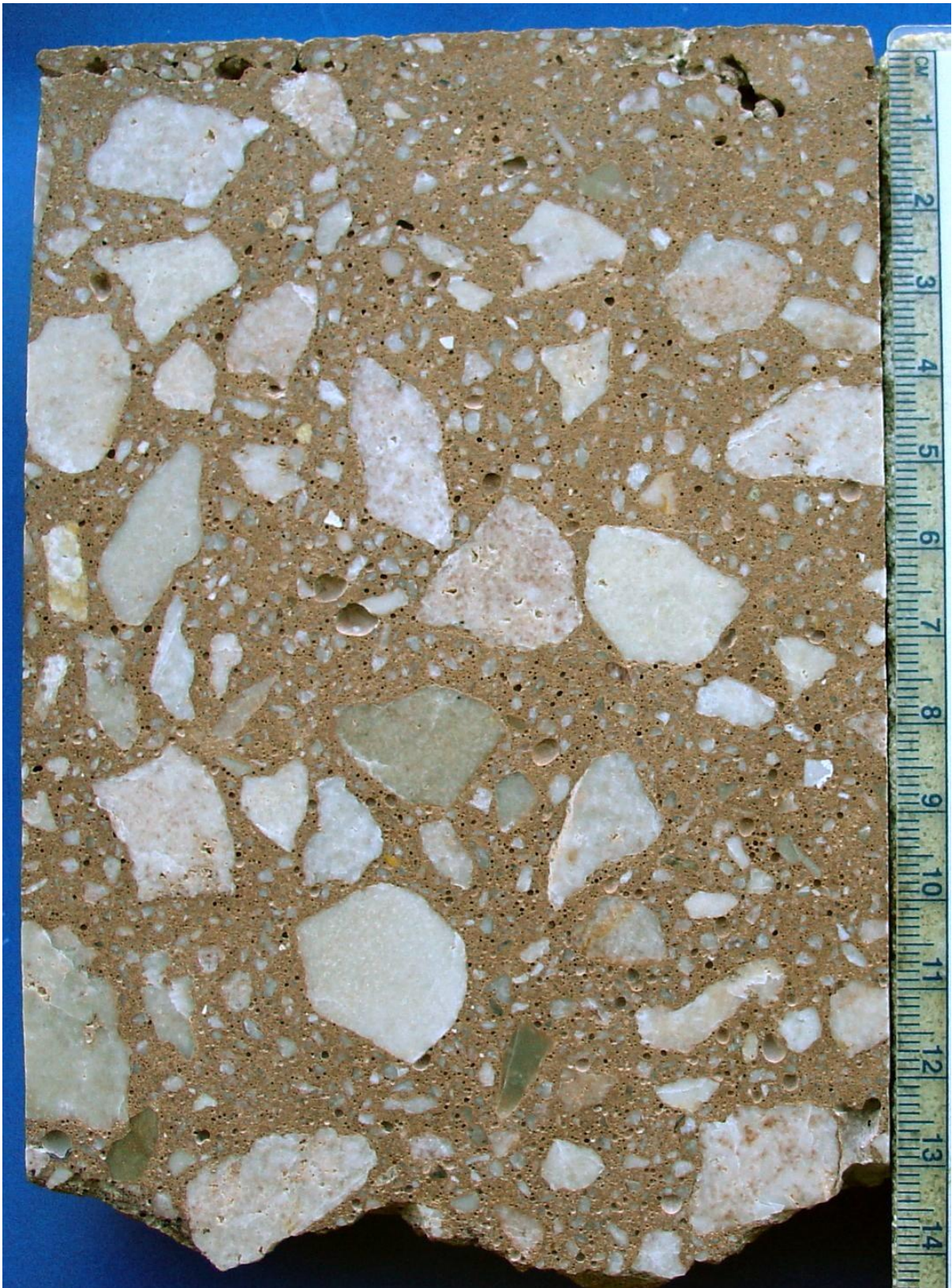
Figure 23. Valley of Fire core #2 with heterogeneous aggregate distribution, abundant entrapped air and crack parallel to the surface on the upper-left that transects entrapped air voids.
