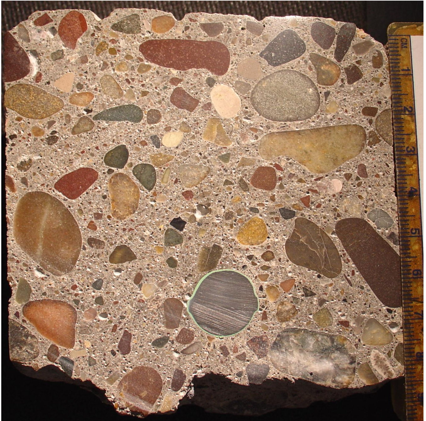
Figure 26. Snake River large-diameter core cross section has a crack extending from one of the surface grooves to the top of the epoxy-coated rebar. Some entrapped air voids are visible.
