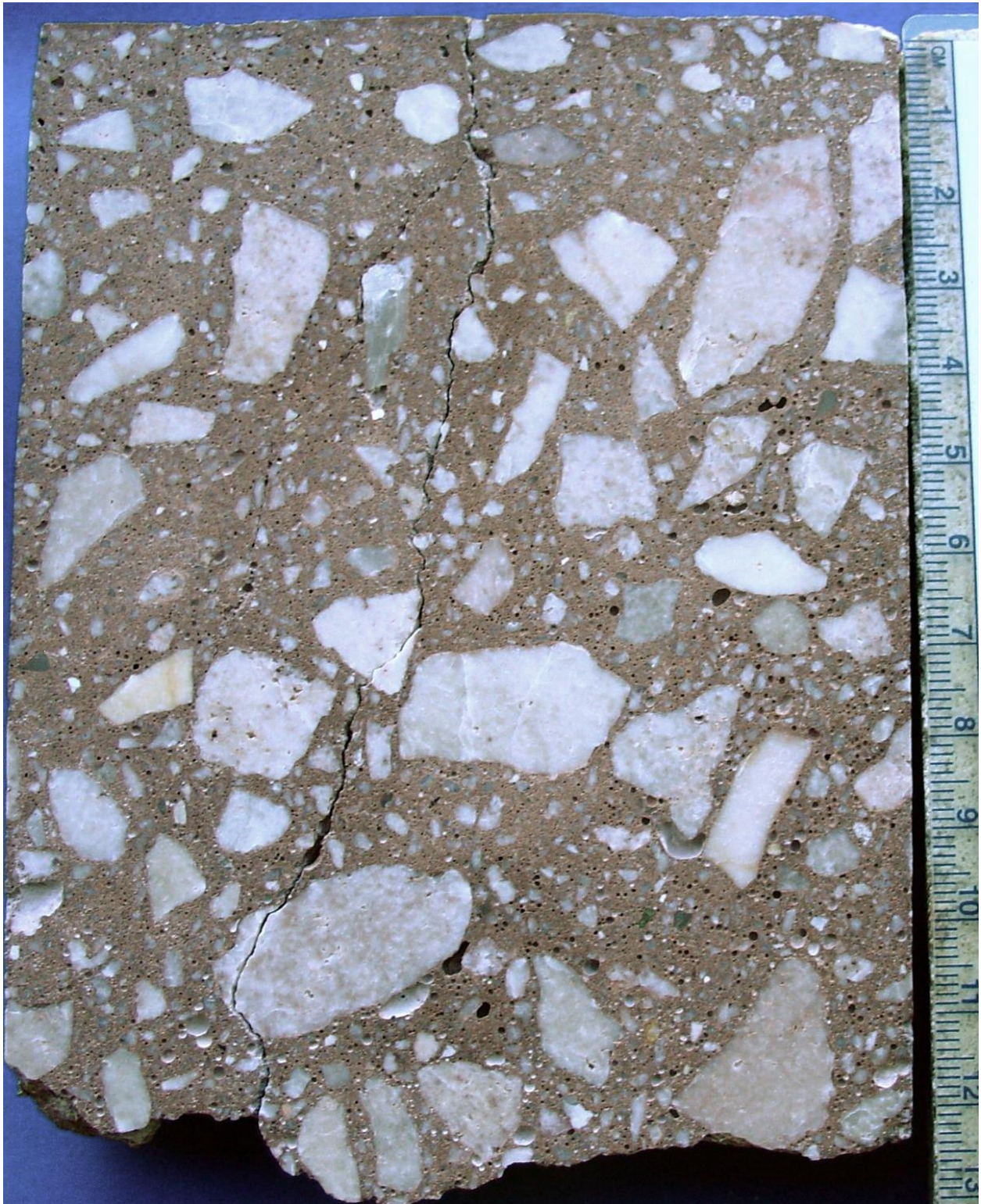
Figure 22. Valley of Fire core #1 with crack extending the length of the section passing mostly through the mortar with a heterogeneous aggregate distribution, common entrapped air, and heterogeneous entrained air void distribution.
