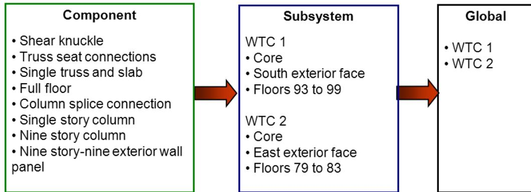
**Figure 2. WTC towers structural analysis sequence [11].**
