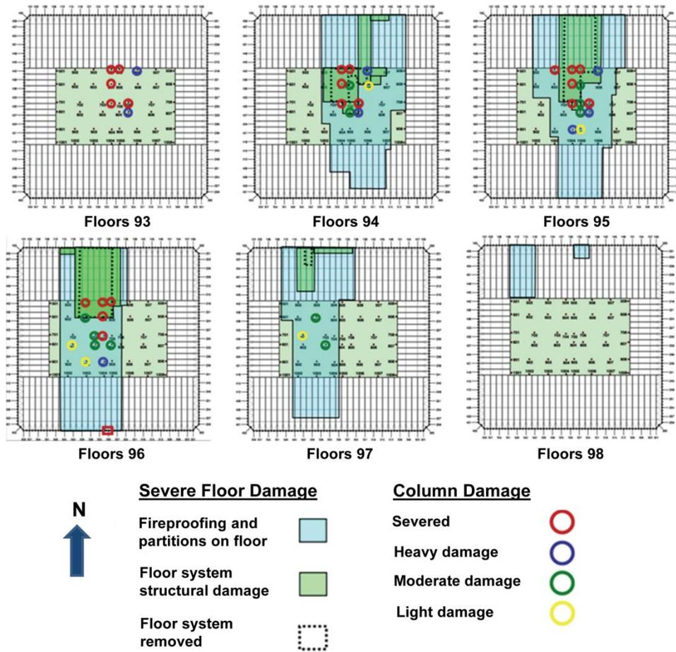
Figure 8. WTC 1 aircraft impact damage based on simulations [11].
