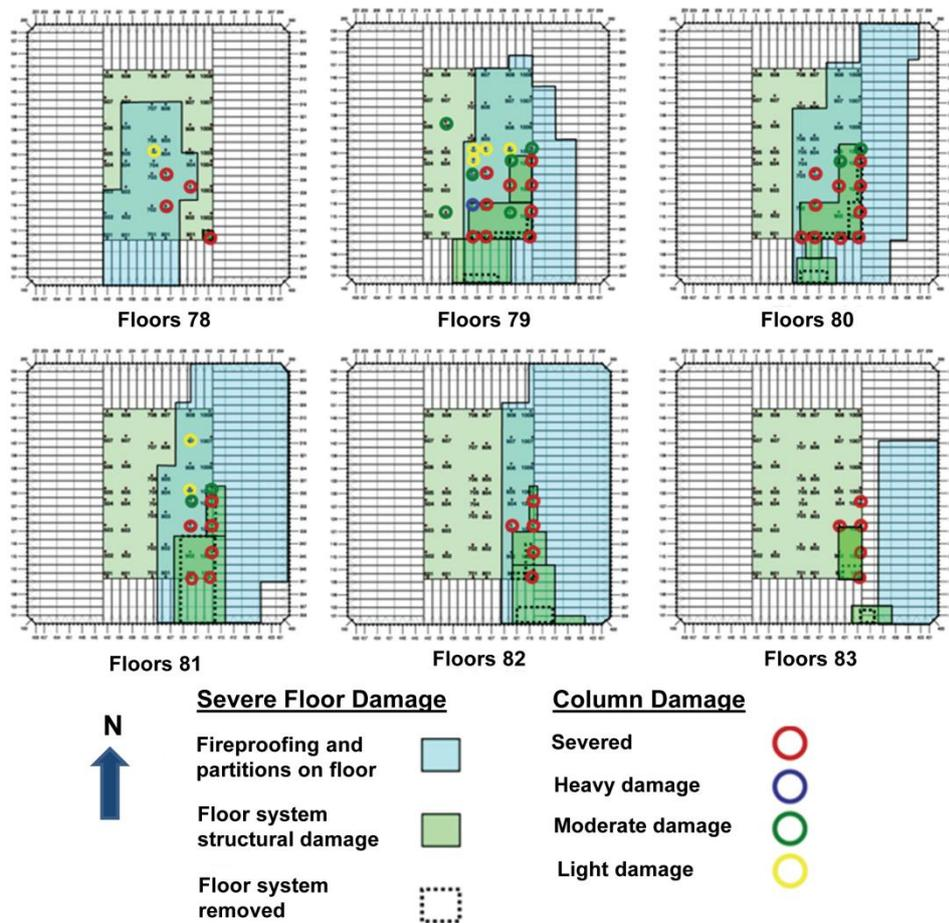
Figure 11. WTC 2 aircraft impact damage based on simulations [11].
