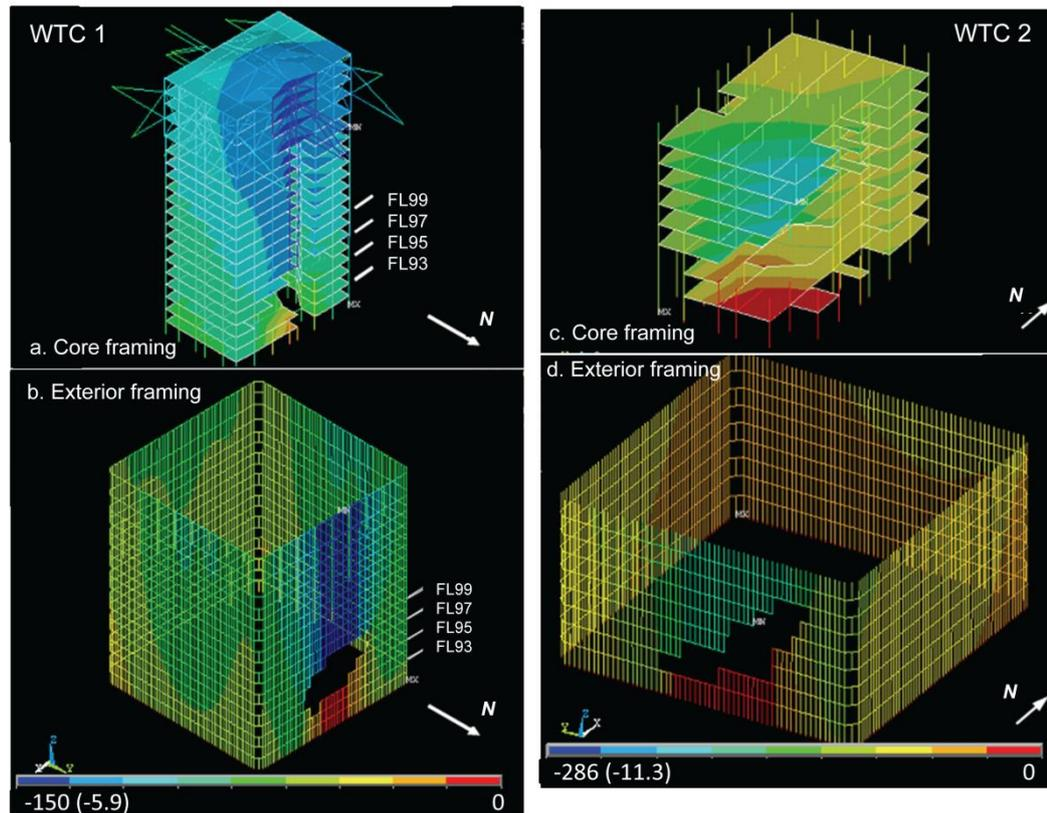
**Figure 9. Vertical displacement in mm (in) based on aircraft impact simulations [11].**
