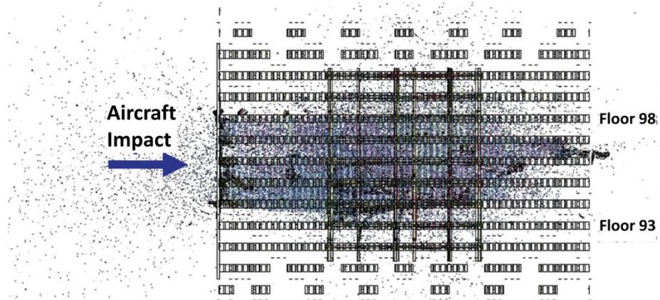
Figure 6. Debris and fuel field in WTC 1 analysis of aircraft impact [27].
