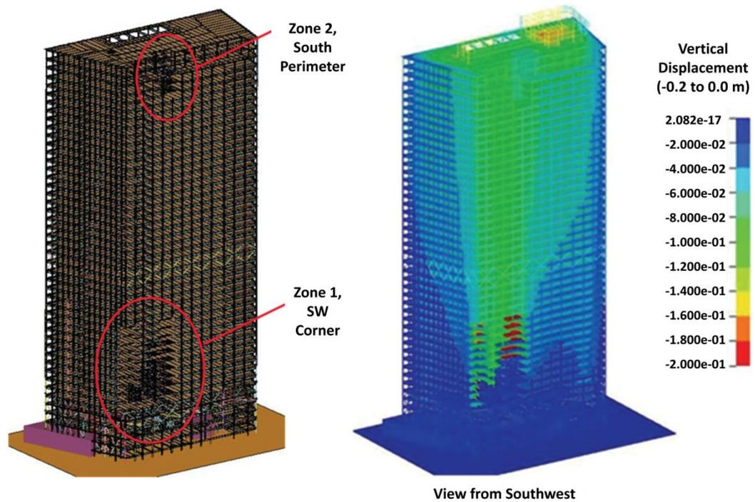
**Figure 12. WTC 1 debris impact damage applied to WTC 7 model (left) and simulated vertical displacement (right) [12].**
