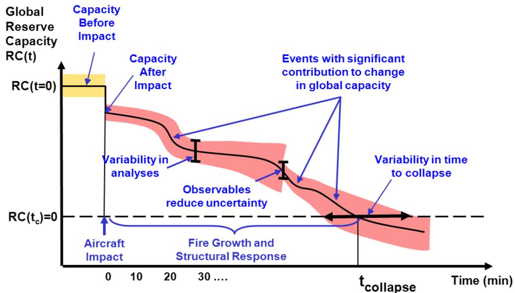
**Figure 3. Schematic of the variability in simulations of global structural capacity using model predictions and observables for sequential analyses with imperfect information [11].**
