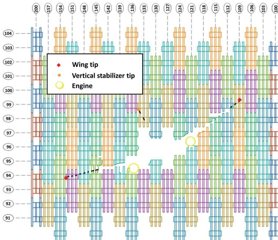
Floor numbers on the left point to the floor slabs. Top numbers refer to exterior columns. The colors distinguish the individual three-column-wide, three-story-tall façade sections.
