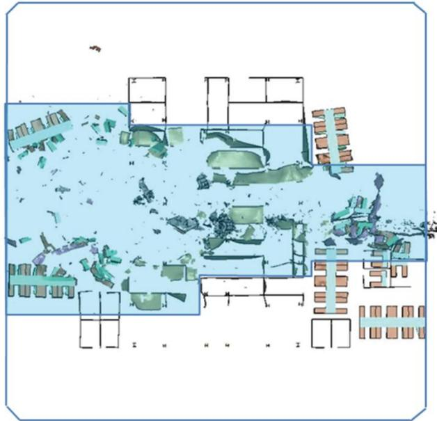
Figure 7. Damage to partitions and furnishings in WTC 1 analysis of aircraft impact to floor 95. Overlay shows extent of estimated dislodged SFRM [11].
