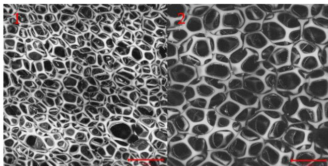
Figure 3. Confocal images for: a smoldering foam (on the left – sample 1 of Fig. 1) and a non-smoldering foam (on the right – sample 2 of Fig. 2). The two foams have an identical formulation but a lower head pressure for foam 1 induces a higher surface area. (Bar size shown is 1 mm).
