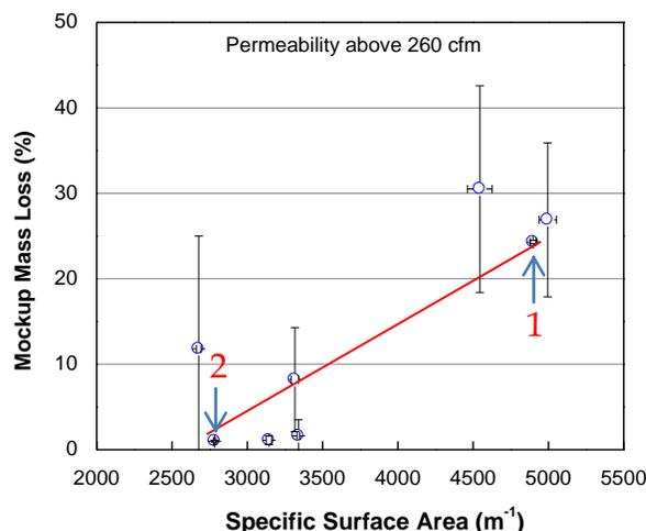
Figure 2. Mockup mass loss vs. specific surface area.
