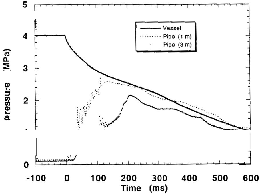
Figure 6. Pressure traces for HFC-227ea tested at a 50% fill condition, pressurized to 4.1 MPa with no make-up nitrogen addition.
