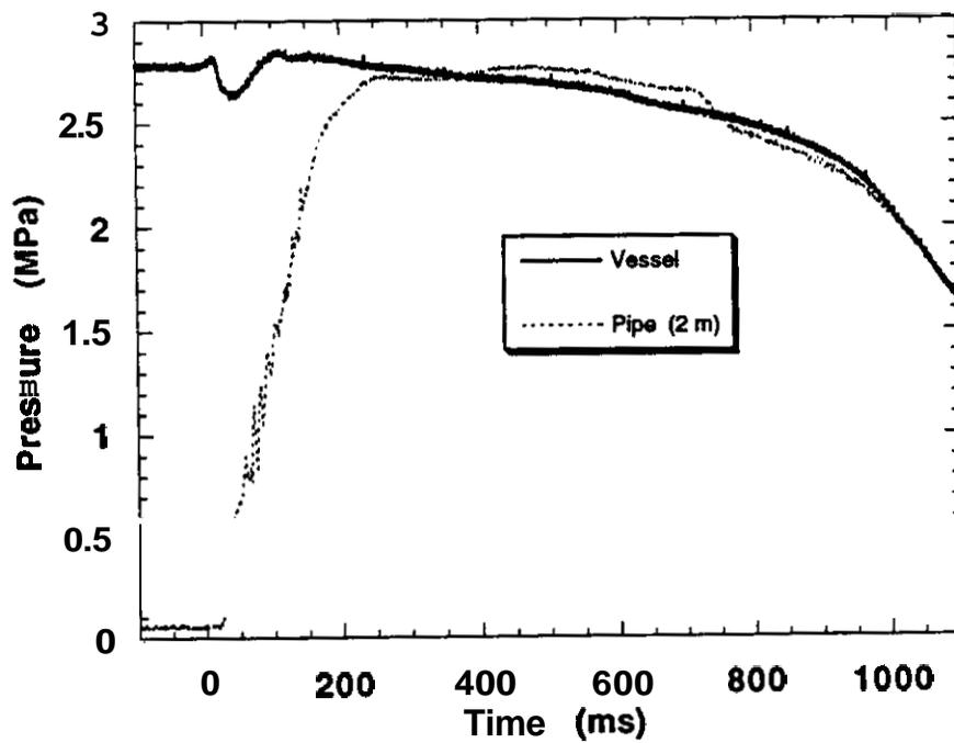
Figure 3. Pressure traces for HFC-227ea tested at a 50% fill condition, pressurized to 2.8 MPa with make-up nitrogen addition.
