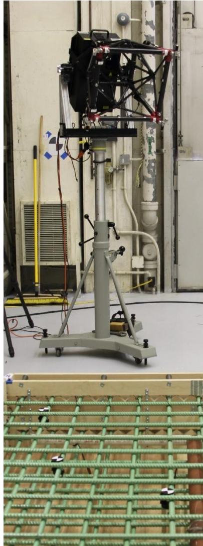
Figure 5-16 The laser projector used to visualize results on the actual rebar.
