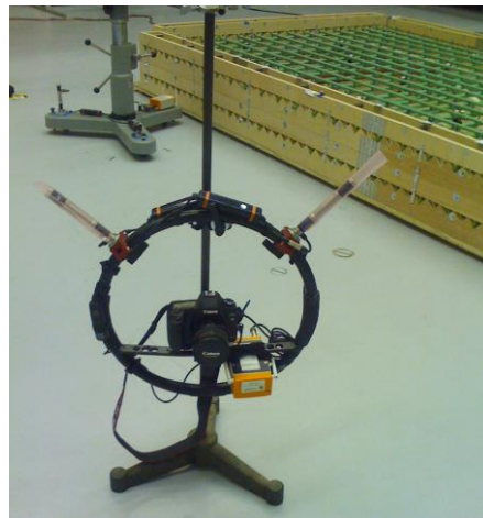
Figure 5-10 The camera with the iGPS receiver frame.
