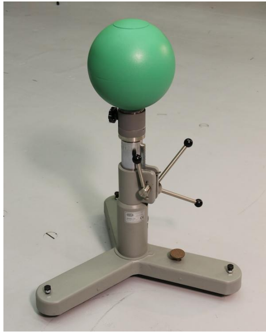
Figure 2-17 The large test sphere used to evaluate the static performance of the CCN.
