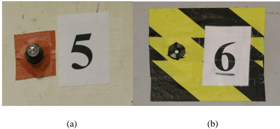
Figure 5-6 Pictures of two IACJS Testbed monuments on the wall (a) and on the floor (b).
