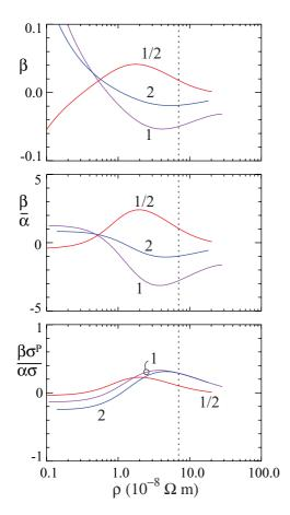
FIG. 5. (Color online) Spin-transfer torque parameter versus resistivity for several ratios (r = 0.5, 1.0, 2.0) of spin-dependent scattering rates for Ni. The top panel gives  $\beta$ , the middle panel  $\beta/\alpha$ , and the bottom panel  $\beta\sigma_{\rm P}/(\alpha\sigma)$ . The dashed vertical lines indicate the approximate room-temperature resistivity.
