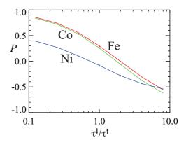
FIG. 2. (Color online) Polarization for bcc Fe (red), hcp Co (green), fcc Ni (blue) as a function of the ratio of lifetimes for the two spin channels,  $r = \tau^{\downarrow}/\tau^{\uparrow}$ . At each value of r, P is calculated for a range of  $\tau^{\uparrow}$  and  $\tau^{\downarrow}$  and the range of resulting values is indicated by the vertical bar at each data point.
