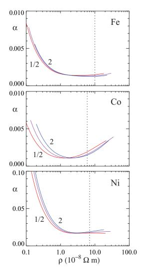
FIG. 3. (Color online) Damping constant versus resistivity for a series of ratios of spin-dependent scattering rates,  $r = \tau^{\downarrow}/\tau^{\uparrow} = 2$ , 1, 0.5. Dashed vertical lines indicate approximate room-temperature resistivities for each element.
