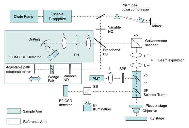
Fig. 1. Optical coherence (OCM)/two-photon fluorescence (2pF) microscope optomechanical diagram. BF: brightfield, BS: beamsplitter, CCD: charge-coupled device, L: lens, ND: neutral density filter, PH: pinhole, PMT: photo-multiplier tube, SPF: short pass filter.
