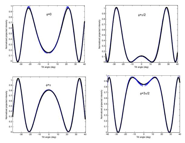
Figure 4. Experimental (thin blue lines) and theoretical (thick black lines) projected intensity of the total field as a function of the QP tilt angle for input phase states  $\phi = \{0, \pi/2, \pi, 3\pi/2\}$ .
