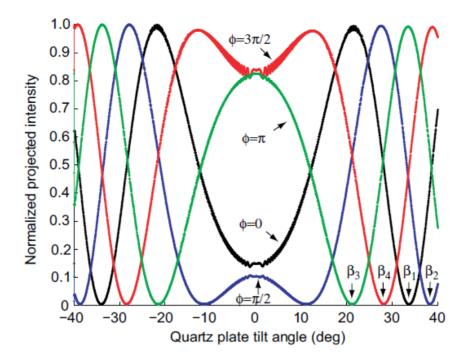
Figure 3. Projected and normalized intensity of the total field containing the signal and LO after the polarizer for input signals in a QPSK format as a function of the QP tilt angle working as a continuous phase shifter.
