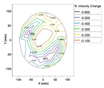
Fig. 3. Composite contour map of the within wafer variation of the change in sound velocity of blanket  $SiO_x$  on a 200 mm wafer.
