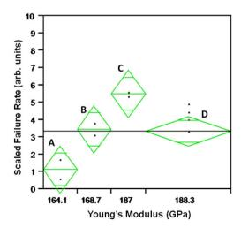
**Fig. 2.** Lot rejection rate as a function of the effective Young's modulus of the encapsulating dielectric stacks for the four different fabrication sites.
