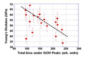
Fig. 4. Correlation of Young's modulus with relative local SiOH concentration from various dies from a typical  ${\rm SiO}_2$  wafer.
