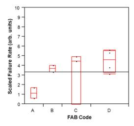
Fig. 1. Lot rejection rate as a function of device fabrication location.
