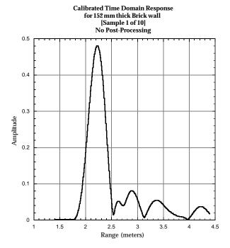
Figure 2.6.2: Calibrated Time Domain Response for 152 mm thick Brick wall (no post processing) for the 0.5 to 2.0 GHz test series, Specimen #1 of 10.
