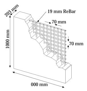
Figure 3.4.2: Reinforced concrete specimen RC881, nominally 203 mm thick, Batch #8 concrete mix with 2% steel.
