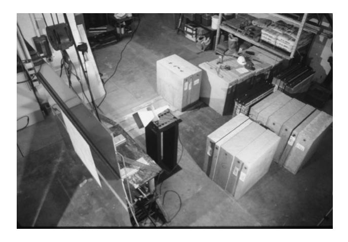
Figure 4.9: Test setup for specimen C612H (305 mm thick plain concrete wall) for frequency response determination from 3.0 to 8.0 GHz.
