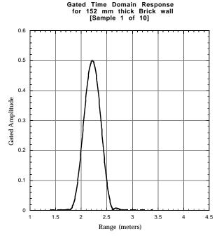
Figure 2.6.3: Gated Time Domain Response for 152 mm thick Brick wall for the 0.5 to 2.0 GHz test series, Specimen #1 of 10.
