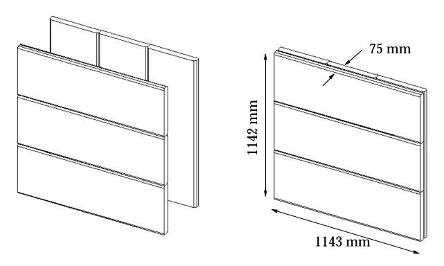
Figure 3.6.2: Specimen L30, a double layer built-up lumber specimen consisting of six "2x12" planks. Both dry and wet speciments were tested.
