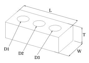
Figure 3.1.1: Individual brick geometry. Definitions of each parameter are given in Table 3.1.2 along with typical measurements and statistical parameters. Individual bricks were used to construct typical residential and commercial building walls of 1,2, and 3 wythe depth, as shown in Figure 3.1.2.
