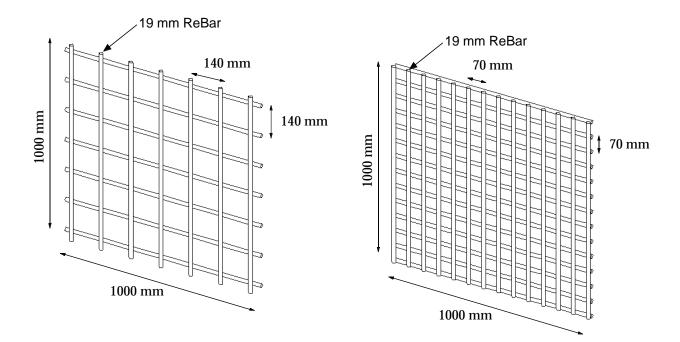
Figure 3.4.3: Bare rebar grid (the same as used in reinforced concrete specimen RC881). Seven 19 mm bars each in the horizontal and vertical directions were used to create a square mesh with 140 mm spacing between bar centers. This left open areas measuring 121 mm square for an open area to solid ratio of 75.2%
