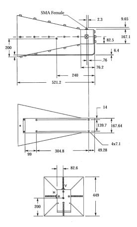
Figure 2.2.2: Side, Bottom, and End Views, top to bottom, respectively, for the WJ-48450, 0.5 to 2.0 GHz antenna (Condor Systems, 1996).
