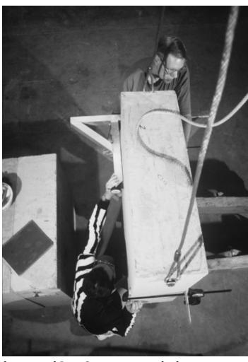
Figure 4.7: Erik Anderson and Jose Ortiz measure thickness sections for 305 mm nominal thickness plain concrete panel.
