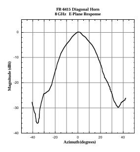
Figure 2.2.2.5: E-Plane radiation pattern for FR-6415 at 8.0 GHz.
