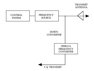
Figure 2.1.2: Simplified schematic of the transmission system and means for characterizing the transmitted signal.
