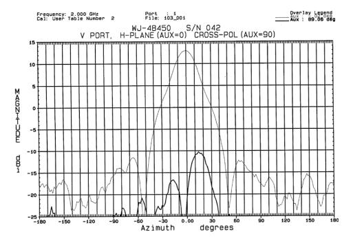
Figure 2.2.7: Typical H-plane radiation pattern (Magnitude in dBi as a function of azimuth angle in degrees) for a WJ-48450 horn operating at the higher, 2.0 GHz, limit of its design spectrum (Condor Systems, 1996).
