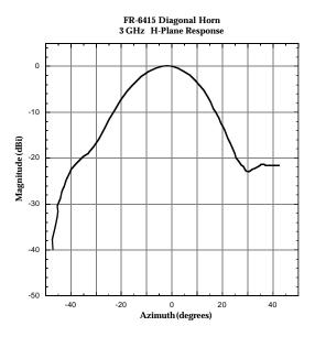
Figure 2.2.2.4: H-Plane radiation pattern for FR-6415 at 3.0 GHz.
