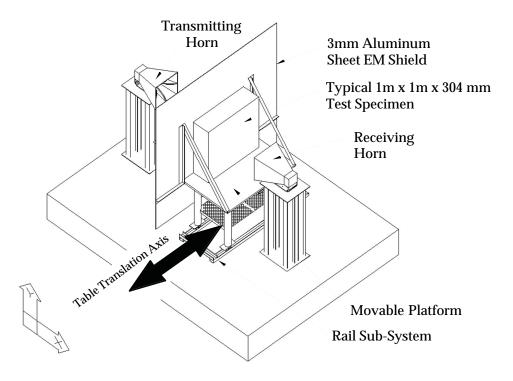
Figure 2.3.1: Isometric view of test stand for Phase 2 NLS tests. Mobile table is shown with specimen in place on opposite side of EM shield from transmitting horn.
