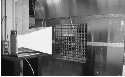
Figure 4.20b: Specimen RE2L (19 mm diameter reinforcing bars on 70 mm centers). Frequency test range: 0.5 to 2.0 GHz. See Figure 5.20a and 5.20b.
