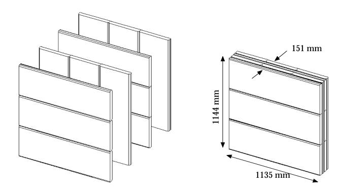
Figure 3.6.4: Specimen L60, a quadruple layer built-up lumber specimen consisting of twelve "2x12" studs. Both dry and wet speciments were tested.
