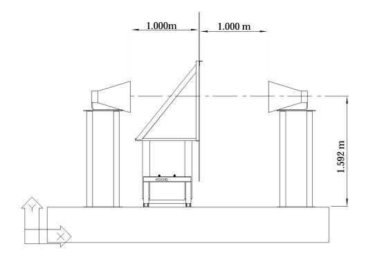
Figure 2.3.5: Elevation view of test stand for Phase 2 NLS tests
