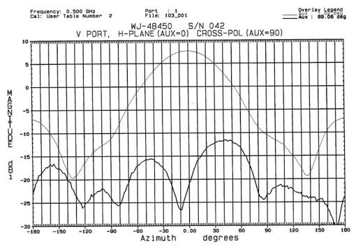
Figure 2.2.5: Typical H-plane radiation pattern (Magnitude in dBi as a function of azimuth angle in degrees) for a WJ-48450 horn operating at the lower, 0.5 GHz, limit of its design spectrum (Condor Systems, 1996).
