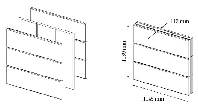
Figure 3.6.3: Specimen L45, a triple layer built-up lumber specimen consisting of nine "2x12" studs. Both dry and wet speciments were tested.
