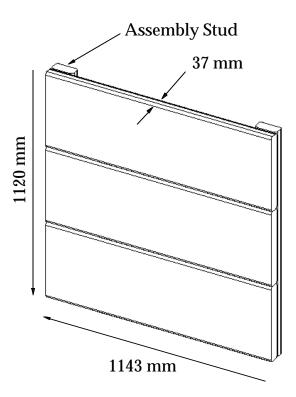
Figure 3.6.1: Specimen L15, a single layer built-up lumber specimen consisting of three "2x12" planks mounted on a "2x4" exterior frame. Both dry and wet speciments were tested.
