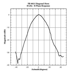
Figure 2.2.2.6: H-Plane radiation pattern for FR-6415 at 8.0 GHz.
