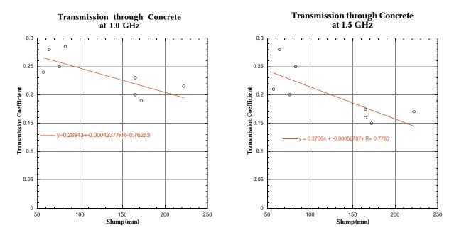
Figure 5.1: Signal attenuation versus slump relationship considering all eight concrete mixtures at two representative discrete frequencies (1.0 and 1.5 GHz) for 102 mm thick plain concrete specimens.
