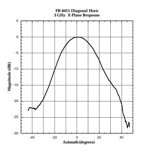
Figure 2.2.2.3: E-Plane radiation pattern for FR-6415 at 3.0 GHz.
