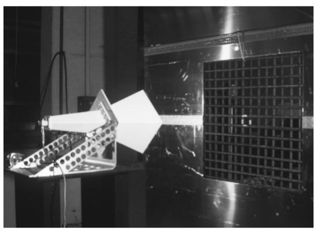
Figure 2.2.2.2: Flam & Russell Diagonal Range Illumination Horn (3.0 to 8.0 GHz) in use with concrete reinforcement grid specimen.
