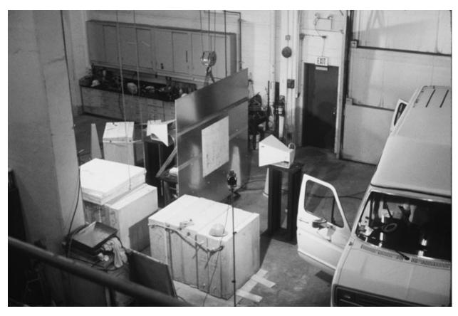
Figure 4.13: Test setup for specimen D25L (nominal 6 mm thick drywall panel) for frequency response determination from 0.5 to 2.0 GHz. See Figures 4.13a and 4.13b.
