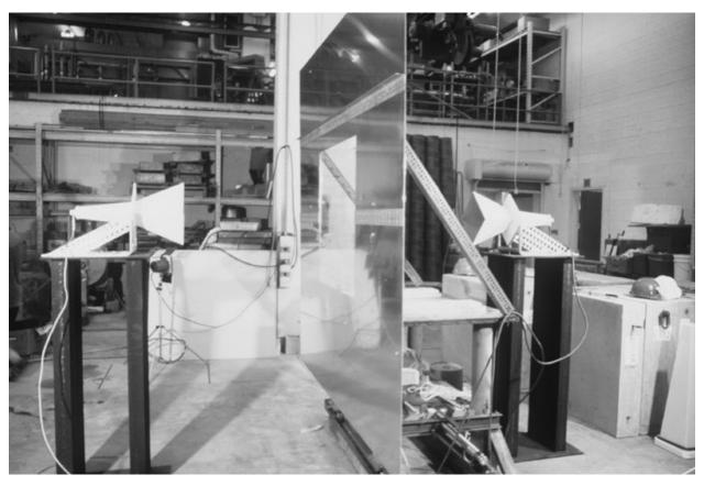
Figure 4.14: Test setup for specimen G75H (19 mm thick silica float glass panel) for frequency response determination from 3.0 to 8.0 GHz. See Figures 4.14c and 4.14d.
