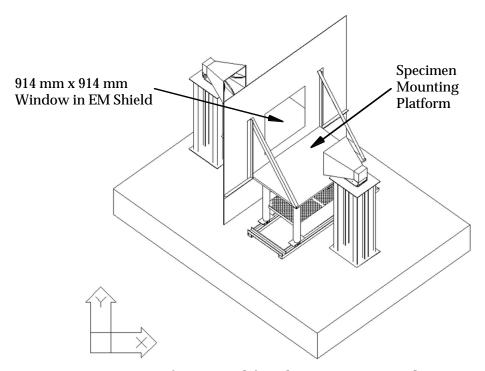
Figure 2.3.2: Isometric view of test stand for Phase 2 NLS tests showing central square window in EM shield.
