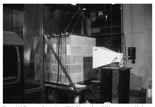
Figure 4.12: Test setup for specimen CB3L (3 layers deep of 203 mm masonry block, total thickness 609 mm) for frequency response determination from 0.5 to 2.0 GHz. See Figures 4.12a and 4.12b.
