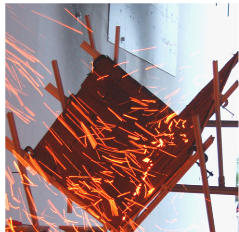
Fig. 7. Fig. 6 OSB base layer, tar paper, and asphalt shingles; angle of 90°–no ignition observed [21]. The wind tunnel speed was 7 m/s. The dimensions of the assembly were 122 cm by 122 cm.
