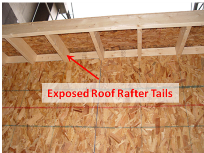
Fig. 16. Image of wall fitted with eave under firebrand bombardment [33]. The wall dimensions were 244 cm by 244 cm with a 61 cm eave overhang.
