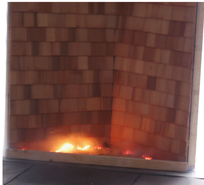
Fig. 14. Images of untreated cedar shingle siding ignited under firebrand attack at a wind tunnel speed of 7 m/s. The dimensions of each side of this assembly were 122 cm wide by 244 cm high.
