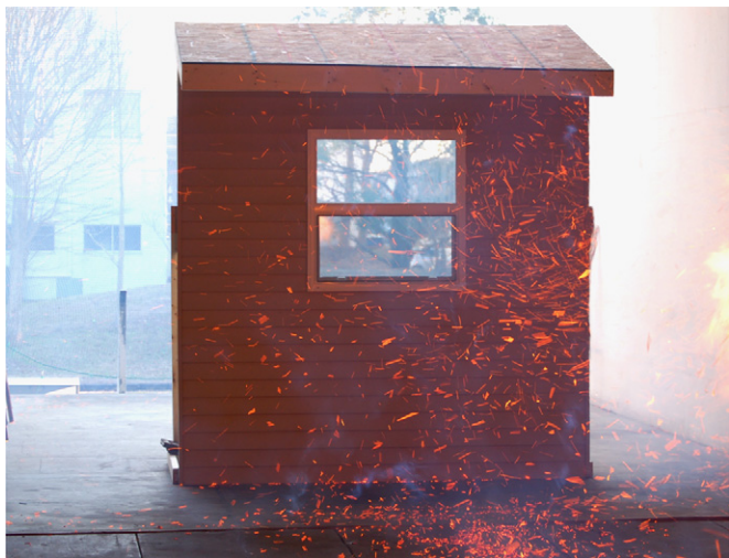
Fig. 18. Picture of wall/eave assembly fitted with a vertically sliding, double hung window exposed to firebrand showers at a wind tunnel speed of 9 m/s [33]. The dimension of wall assembly was 244 cm by 244 cm.
