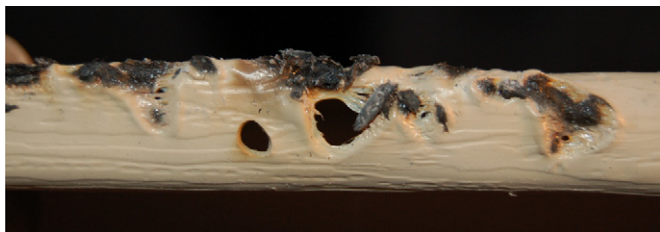
Fig. 12. Image of vinyl siding (from bottom) after firebrand exposure at 7 m/s [33].
