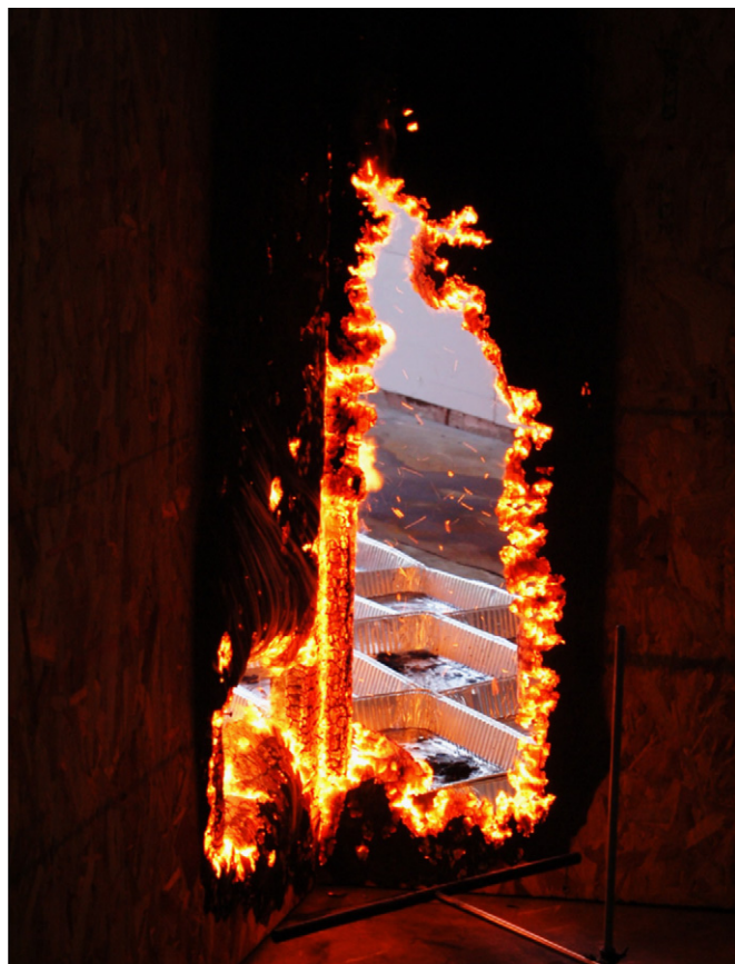
Fig. 22. Firebrand generation from a burning reentrant corner at 8 m/s applied wind [45]. Firebrands are produced on the backside of the assembly and are collected using an array of water pans downstream. The dimensions of each side of the reentrant corner were 122 cm by 244 cm.
