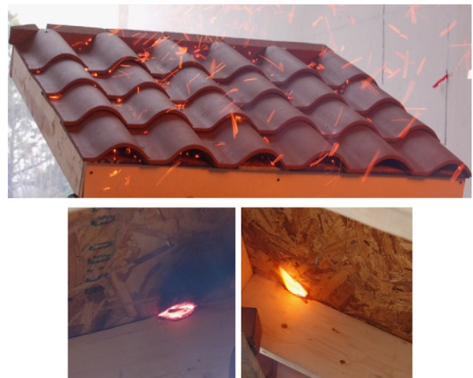
Fig. 5. Images of experiments conducted using OSB/CT without bird stops installed [22]. Intense SI was observed within the OSB base layer and eventually FI was observed. The wind tunnel speed was 7 m/s and the Firebrand Generator was located 2.0 m from the CT roofing assembly. The dimensions of the roof assembly were 122 cm by 122 cm.
