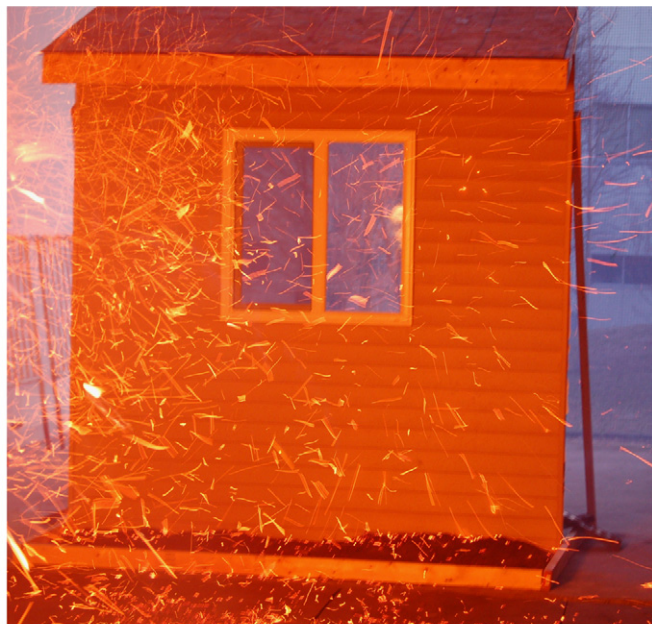
Fig. 12. Image of vinyl siding (from bottom) after firebrand exposure at 7 m/s [33].
