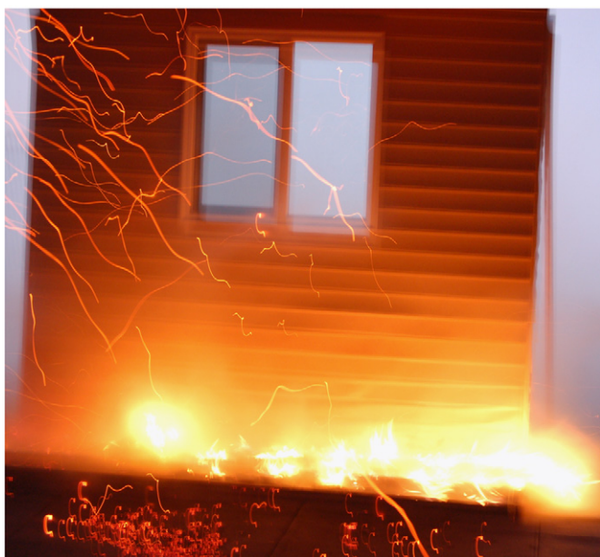
Fig. 13. In the top image, firebrands have caused smoldering ignition in the mulch bed [33]. In the bottom image, smoldering ignition has transitioned to flaming ignition and the wall assembly has ignited. The dimensions of the wall assembly were 244 cm by 244 cm.
