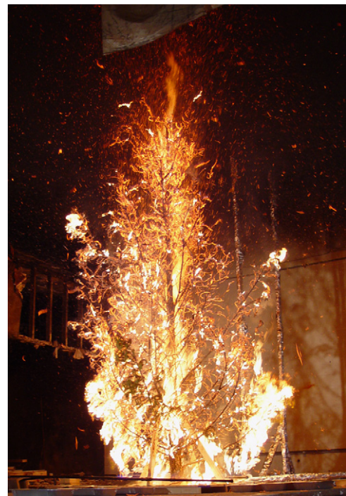
Fig. 3. Photograph of a burning Douglas-Fir tree (5.2 m) used for firebrand collection [25]. This experiment was conducted at NIST's Large Fire Laboratory (LFL).
