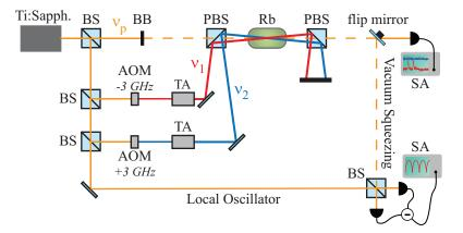
Fig. 2. Experimental setup. AOM: acousto-optic modulator, TA: semiconductor tapered amplifier, SA: radio frequency spectrum analyzer, BS: non-polarizing beamsplitter, PBS: polarizing beamsplitter, BB: beam block. The beam block and the flip mirror are removed in order to seed the 4WM process and permit direct intensity detection with a single photodiode.
