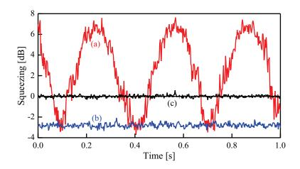
Fig. 4. Vacuum squeezing measured by homodyne detection at 1 MHz when (a) the phase of the local oscillator (LO) is scanned and (b) when the phase of the LO is locked. Trace (c) indicates the standard quantum limit. (RBW = 30 kHz, VBW = 100 Hz.) Comparison of the traces shows a squeezing level of  $(-2.8 \pm 0.2)$  dB. Here  $\Delta = 0.8$  GHz,  $\delta = -4$  MHz, the power in pump 1 is 230 mW and the power in pump 2 is 160 mW.
