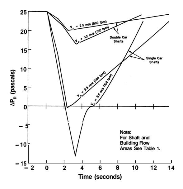
Figure 2. Calculated pressure differences across elevator lobby doors due to piston effect of a single car moving in an eleven story shaft
