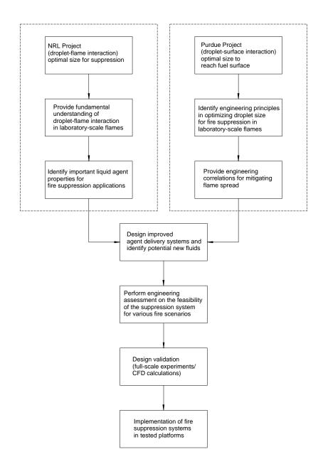
Figure 1. A flowchart showing an overall approach to improve liquid delivery systems.
