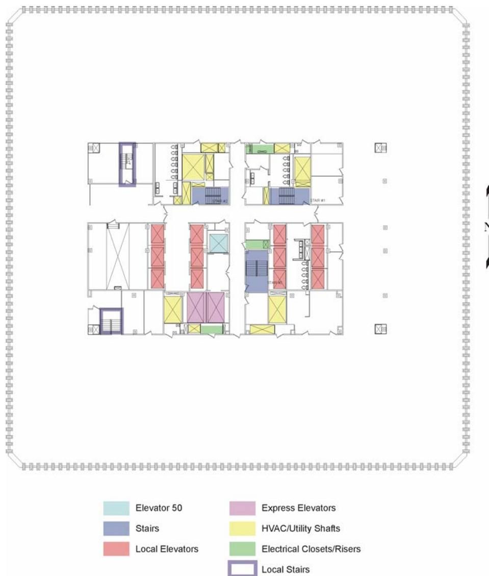
**Figure 4–1. Floor layout, 95th floor, WTC 1.**
