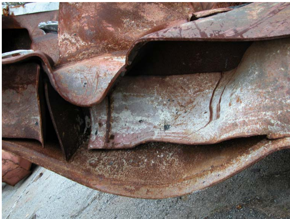
Figure 2–16. Photograph of an exterior column with weld zone fractures.
