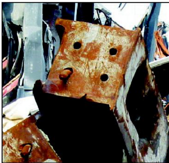
Figure 5–10. Failure behavior observed in the external column bolted joints.
