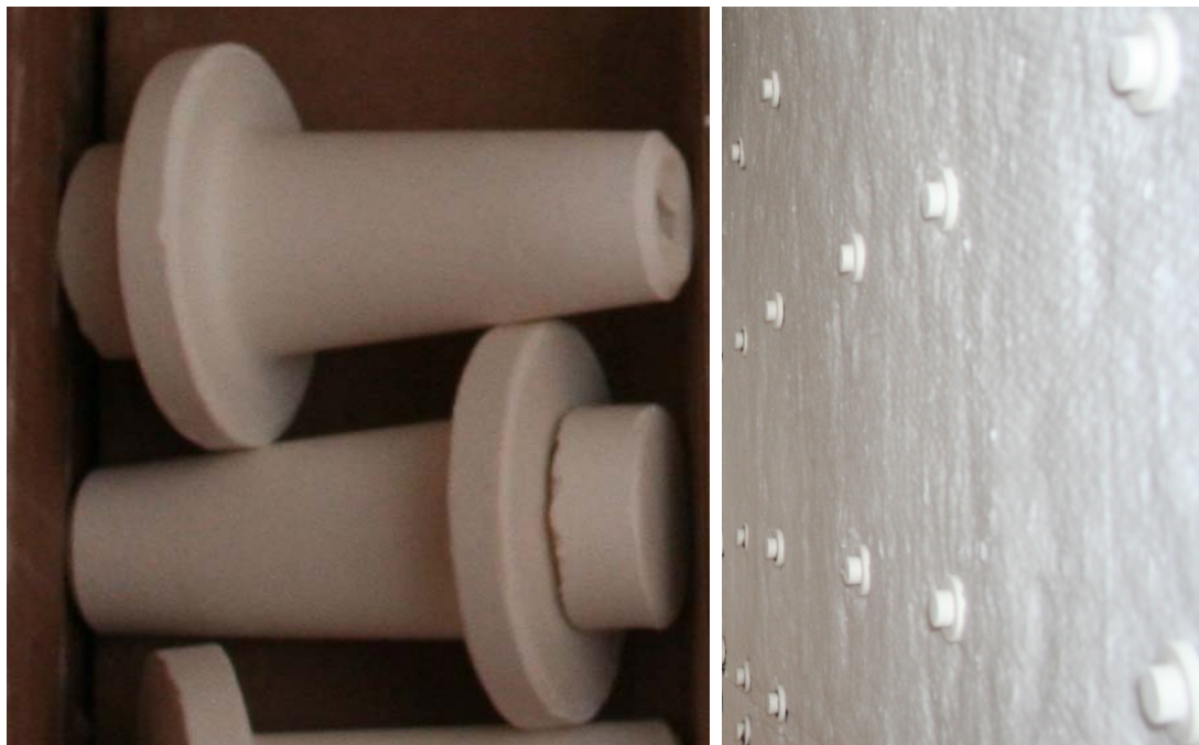
Figure 2.3 Ceramic insulation retainers used to secure the ceramic fiber blanket to the sheet steel walls. The actual retainer is shown (left) as well as its installed configuration (right).
