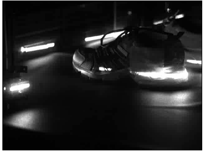
Video 8. Particle release from the outer heel. The laser light sheet has a vertical orientation.
