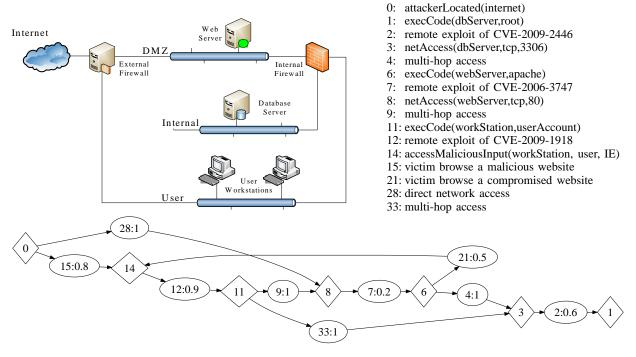
Figure 1. Example scenario and attack graph
