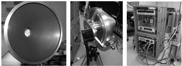
**Figure 2.** Inside of the optical cavity showing the black coating (left), front view of the BB Prime (center), and portable, modular control equipment (right).
