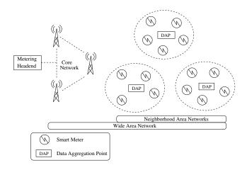
Fig. 1. Metering network topology
