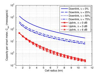
Fig. 7. Smart meter capacity in rural environment with 8 dB shadowing
