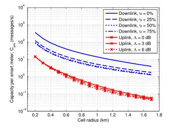
Fig. 6. Smart meter capacity in urban environment with 8 dB shadowing
