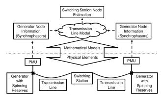
Fig. 1. Schematic representation of the coupled interaction between physical elements and mathematical elements discussed in the use case. PMUs serve as the interface between the two domains.
