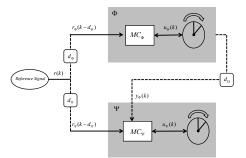
Fig. 2. A schematic showing the control layout for the networked masterslave pair. The blocks  $d_{\Phi}$ ,  $d_{\Psi}$ , and  $d_{\Omega}$  symbolize network delays between the respective components.  $MC_{\Phi}$  and  $MC_{\Psi}$  are the motor controllers.  $y_{\Phi}(k)$  is the trajectory of  $\Phi$ : and  $u_{\Psi}(k)$  and  $u_{\Phi}(k)$  are the control signals sent to the motors.  $\Phi$ : and  $\Psi$  denote the two individual dynamic systems.
