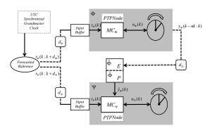
Fig. 3. A schematic of the same control layout shown in Figure 2. Modules E and P denote the Estimation and Propagation blocks added to compensate for delays  $d_{\Phi}$ ,  $d_{\Psi}$ , and  $d_{\Omega}$ .
