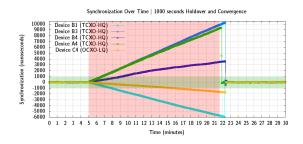
Fig. 4. A plot of the drift upon loss of connection to the Grandmaster and resynchronization of PTP slave devices. Note the large variation in performance.
