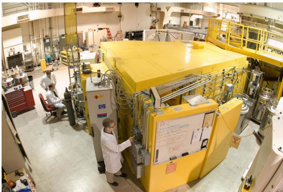
NCNR's David Jacobson stands before the Neutron Imaging Facility that has played a unique role in revealing the flow of product water during the operation of fuel cells being developed by the automotive industry for alternative vehicles. NCNR's Dan Hussey (seated) and Eli Baltic are at the controls at the left. This facility was developed in a partnership between NIST and GM, and is available for use by other U.S. researchers.
