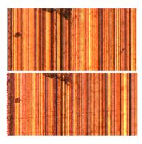
Fig. 2. Two images captured on the same area of the SRM 2460-001 bullet by the same microscope under different lighting directions. (Top) - Area aligned perpendicular to microscope optical axis, (Bottom) – The same area tilted by approximately  $6^{\circ}$ .
