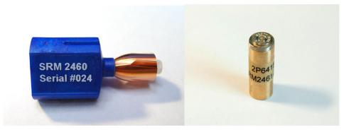
Fig. 1. A SRM 2460 Standard Bullet (left) and a SRM 2461 Standard Cartridge Case (right).
