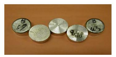
Semi-chill cast disks of SRM 1728 showing various stages in manufacturing and testing.
