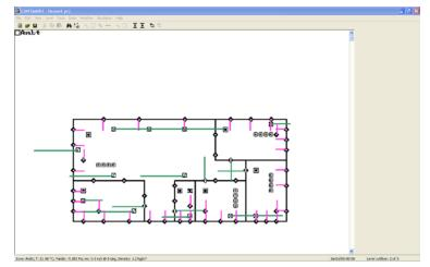
**Figure 2** Airflow simulation result for the model (air flows = green lines, pressure drop = red lines).
