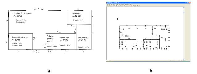
Figure 1 Building floor plan and CONTAM model of the simulated building.
