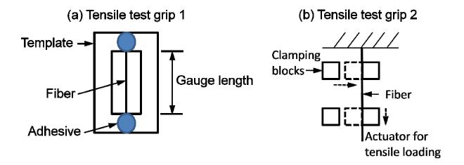
Figure 1 Schematic and closed up of the mechanical grips for single fiber tensile loading.
