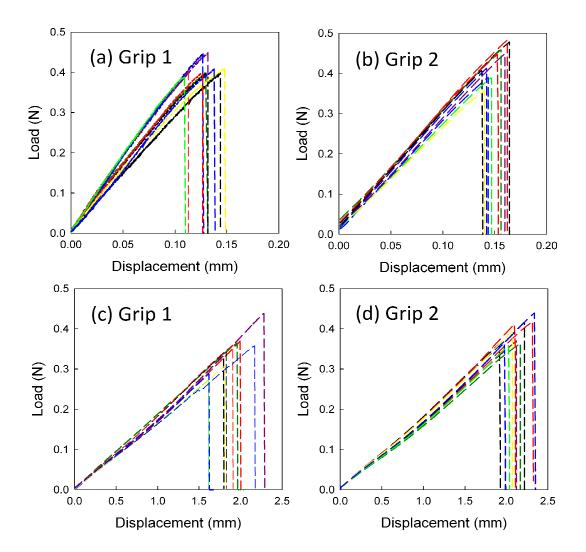
Figure 2 load-displacement curves with 2 mm gauge length (a, b) and 60 mm gauge length (c, d).
