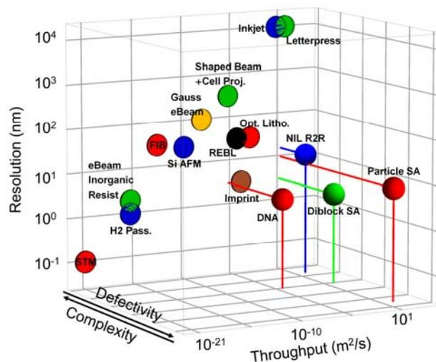
**Figure 2.** Resolution versus throughput and complexity/defectivity for top-down and directed self-assembly fabrication techniques. (R2R is used to denote roll-to-roll processes).
