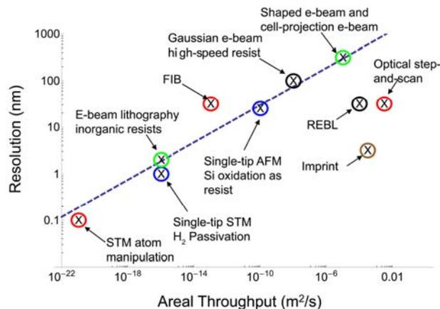
**Figure 1a.** Resolution versus throughput for a variety of top-down lithographic techniques. The blue line is  $3 \times 10^3\text{ nm} \times (\text{Throughput}/(\text{m}^2/\text{s}))^{0.2}$  and corresponds to the best-fit line from the Marrian and Tennant paper. (REBL stands for reflection e-beam lithography)
