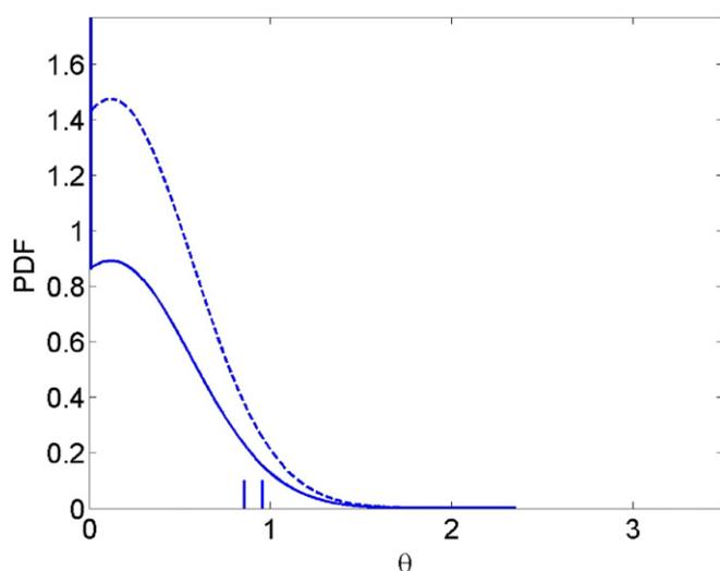
**Figure 5.** GUM-S1 PDF (solid line) and Bayesian posterior (dashed line). The bar at  $\theta = 0$  indicates the discrete part of the GUM-S1 distribution with  $P(\theta = 0) = 0.40$ . The two bars on the abscissa show the upper bound  $\bar{\theta}$  of 95% credible intervals of the form  $[0, \bar{\theta}]$  for the GUM-S1 PDF (left bar at  $\bar{\theta} = 0.85$ ) and the Bayesian posterior (right bar at  $\bar{\theta} = 0.95$ ).
