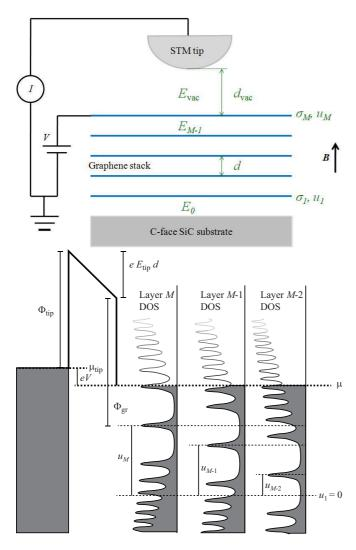
FIG. 4: (color online). Upper panel shows schematic illustration of a few-layer-graphene system with an STM tip. The buffer layer between the SiC and the graphene layers was omitted for simplicity. Lower panel is the energy level diagram for this system.
