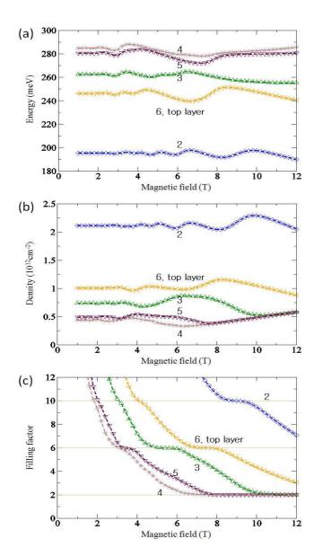
FIG. 8: (color online). Electrostatic energy, density and filling factor of each layer as a function of magnetic field for  $\Phi=400$  meV,  $\mu=360$  meV and T=30 K at zero tip-sample bias voltage. The filling factor of the bottom layer (not shown) exceeds  $\nu=12$  over the field range considered. Numbers indicate layer numbers, with 6 being the topmost layer.
