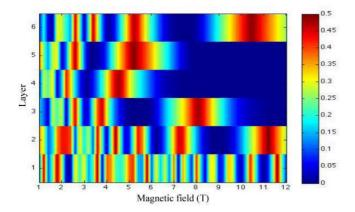
FIG. 10: (color online). Filling factor modulus  $\nu_i^{mod}$  as a function of magnetic field for  $\Phi=400$  meV and  $\mu=360$  meV at T=30 K, where  $\nu_i^{mod}=|(\nu/4 \bmod 1)-1/2|$ . Note that  $\nu_i^{mod}=0$  for  $\nu_i{=}\pm 2,\pm 6,\pm 10,\cdots$ , while  $\nu_i^{mod}=1/2$  for  $\nu_i{=}0,\pm 4,\pm 8,\cdots$ . The points were evaluated at zero bias voltage.
