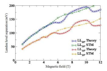
FIG. 9: (color online). Landau level separations between N=0 and the N=1 (N=2), denoted as  $\mathrm{LL}_{10}$  ( $\mathrm{LL}_{20}$ ) for theoretical calculations and STM measurements. <sup>15</sup> For the theoretical calculations,  $\Phi=400$  meV and  $\mu=360$  meV at T=30 K were used.
