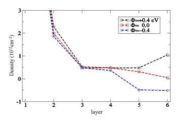
FIG. 5: (color online). Charge density in the layers of a six layer stack at  $B=10\,\mathrm{T}$  for  $\Phi=+0.4\,\mathrm{eV},\,0\,\mathrm{eV},\,-0.4\,\mathrm{eV}$  when the tip-sample bias is zero. These curves were obtained using  $\mu=360\,\mathrm{meV}$  and  $T=30\,\mathrm{K}$ . By construction, electrons have a positive carrier density, while holes have negative density (see text for details).
