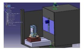
Figure 3: Machining simulation model of MAKINO A55
