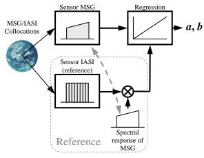
**Figure 2:** Existing calibration scheme of MSG sensors against IASI. The spectral convolution is "matched" to the individual MSG sensor.
