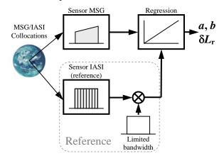
**Figure 3:** Proposed calibration scheme for MSG sensors against a polar-orbiting sensor (IASI). The spectral convolution is reduced to limit the bandwidth.  $\delta L_r$  is an additional component to describe the *Spectral Mismatch* and its uncertainty.
