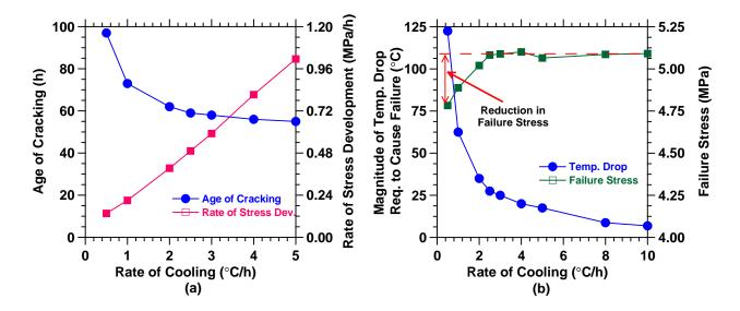
**Fig. 12.** Influence of the rate of cooling on (a) the stress development and the age of cracking, and (b) the magnitude of temperature reduction and the average stress at failure in the dual ring test.
