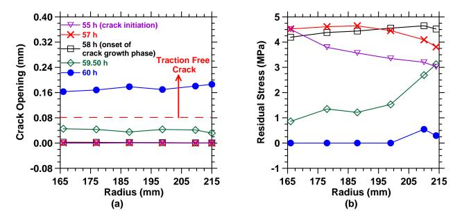
**Fig. 6.** (a) Crack opening displacement and (b) average residual stress profile in the reduced strength section of the base case ring specimen when cooled at 48 h.
