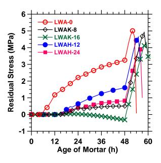
**Fig. 7.** Calculated residual stress development in dual-ring specimens when cooling began after 48 h.
