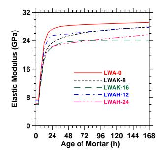
Fig. 2. Elastic modulus development of mortar mixtures (fitted) [23]
