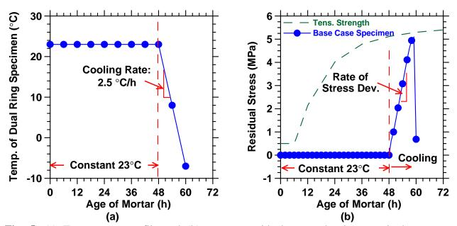
**Fig. 5.** (a) Temperature profile and (b) average residual stress development in base case specimen when cooled at 48 h.
