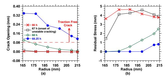
**Fig. 9.** (a) Crack opening displacement and (b) residual stress development through the specimen wall in the damage zone when the elastic modulus was reduced by 60 %.
