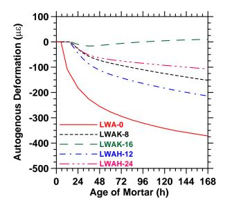
**Fig. 4.** Fitted autogenous shrinkage development of plain mortar and mortars with the pre-wetted LWAs [23]
