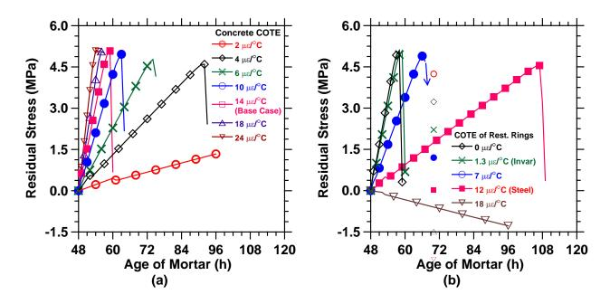
**Fig. 10.** Influence of (a) COTE of the mortar specimen and (b) COTE of restraining rings on the average residual stress development.
