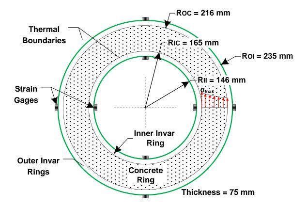
Fig. 1. Schematic overview of the finite element model
