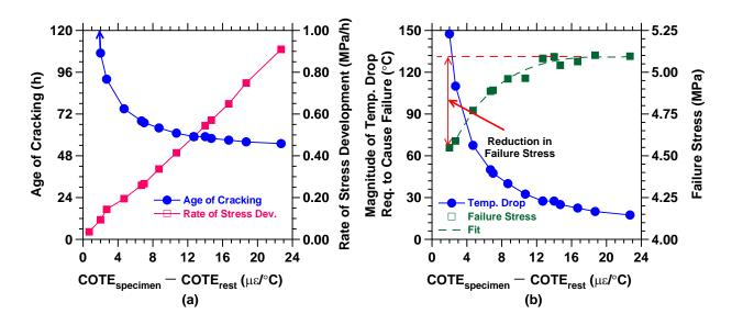
**Fig. 11.** Influence of relative thermal deformations of the mortar and restraining rings on (a) the rate of stress development, age of cracking, (b) the magnitude of temperature drop, and the reduction in average stress of dual ring specimen at failure.
