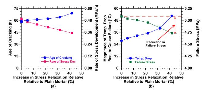
**Fig. 13.** Influence of stress relaxation on (a) the stress development and the age of cracking, and (b) the magnitude of temperature reduction and the average stress at failure in the dual ring test.
