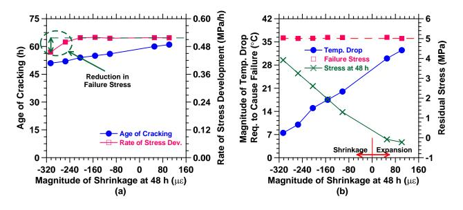
Fig. 14. Influence of autogenous shrinkage on (a) the stress development and the age of cracking,(b) the magnitude of temperature reduction, stresses at 48 h, and the average section stress at failure in dual ring test.
