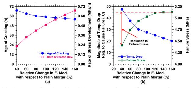
**Fig. 8.** Influence of elastic modulus of the specimen on (a) the residual stress development, age of cracking, (b) the magnitude of temperature drop, and the reduction in strength.
