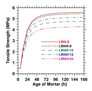
Fig. 3. Tensile strength development of mortar mixtures (fitted) [23]
