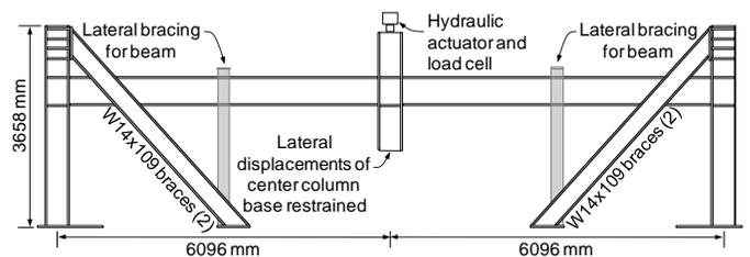
Figure 2. Test setup for the steel assembly.
