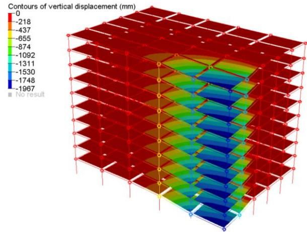
Figure 17. Vertical displacements from pushdown analysis of concrete IMF building with three missing columns.
