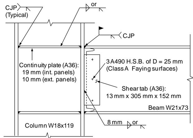
Figure 1. WUF-B connection details for the steel assembly.
