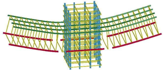
Figure 14. Failure mode from detailed model of the reinforced concrete assembly.
