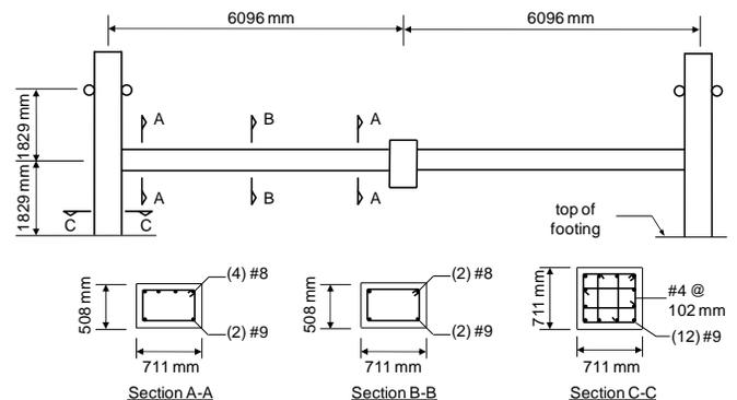
Figure 8. Schematic of the reinforced concrete assembly.
