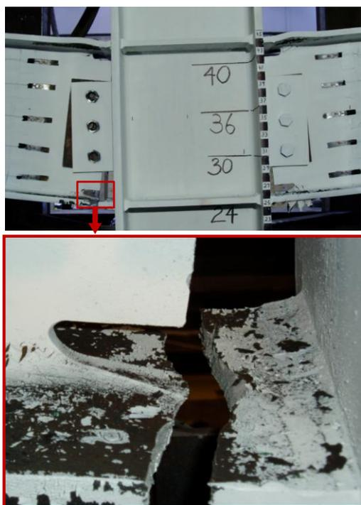
Figure 4. Failure mode of the steel assembly.
