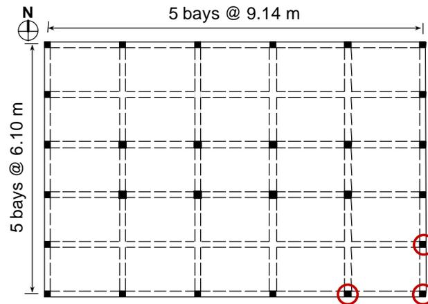
Figure 18. Plan layout of concrete IMF building. Circles indicate columns removed prior to pushdown.
