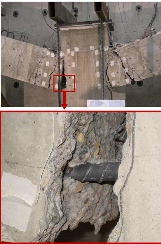
Figure 12. . Failure mode of the reinforced concrete assembly.
