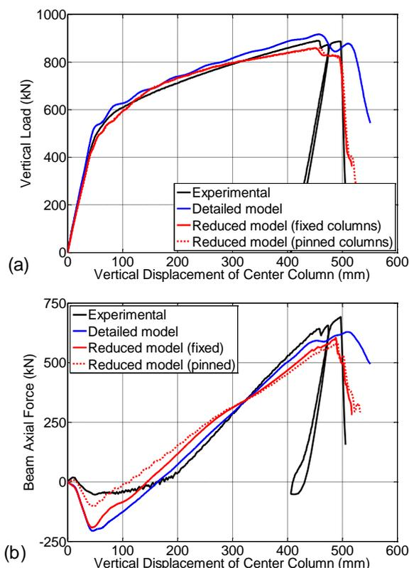
Figure 5. (a) Vertical load and (b) beam axial force versus vertical displacement of center column for the steel assembly (measurement uncertainty:  $\pm 1\%$ ).
