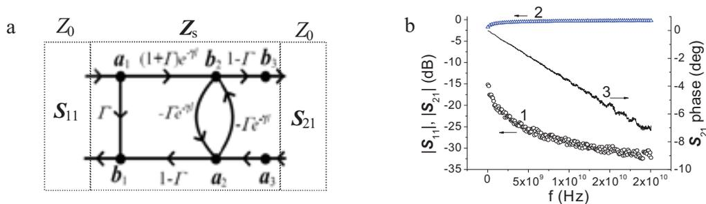
FIGURE 1. a- Signal flow graph of CPW. b- Scattering parameters for Au film. (1)- $|S_{11}|$ , (2)-  $|S_{21}|$  and (3) - phase of  $S_{21}$ .
