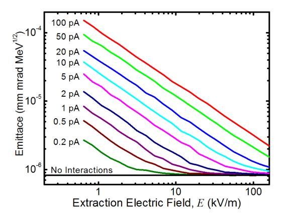
FIG 5. Monte Carlo simulated beam emittance for selected currents as a function of extraction electric field E. MOTIS geometry and temperature of the source are the same as in Figs. 1-3. At higher currents and at lower extraction electric fields the final emittance after being accelerated over 6 mm is larger than the interaction-free value. However, for a sufficiently high extraction field, all beam currents converge to the interaction-free emittance value.
