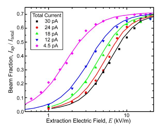
FIG 6. Fraction of beam current passing a 20  $\mu$ m aperture vs extraction electric field for various beam currents. Symbols are experimental data and solid lines are Monte Carlo simulations. Uncertainties of the measured data are  $\pm$  7 %.
