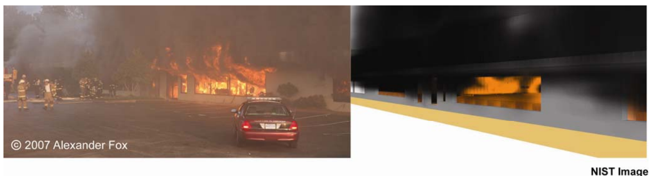
Figure 4-22. Comparison between photo and rendered image from the simulation at 1655 s (7:38:28 p.m.). The view is of the front of the main showroom.
