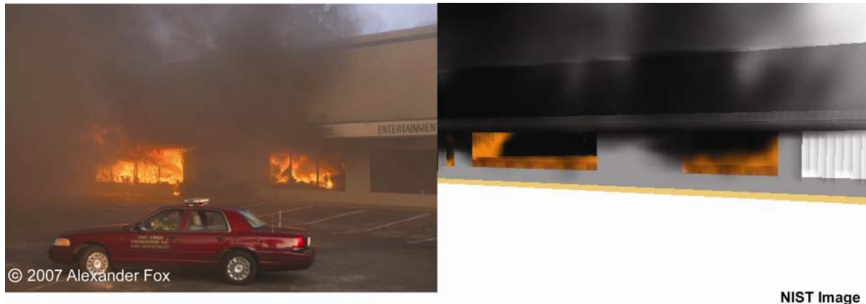
Figure 4-23. Comparison between photo and rendered image from the simulation at 1686 s (7:38:59 p.m.). The view is of the front of the main and west showrooms.
