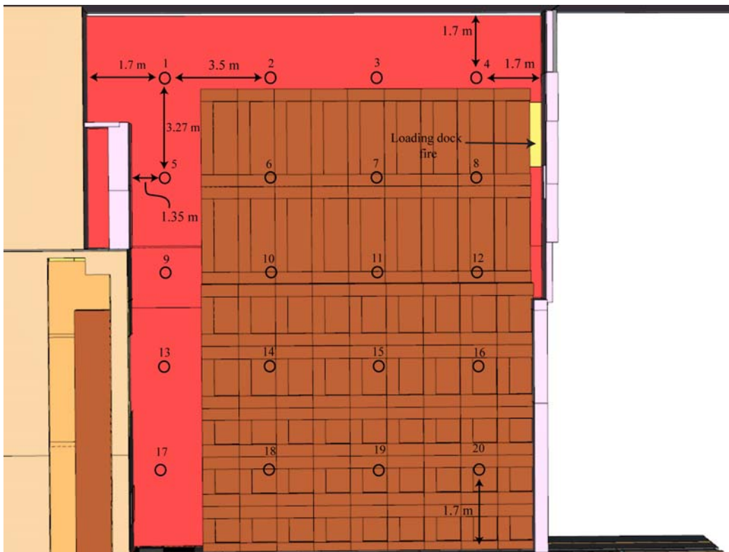
Figure 4-35. Sprinkler layout inside the enclosed loading dock.
