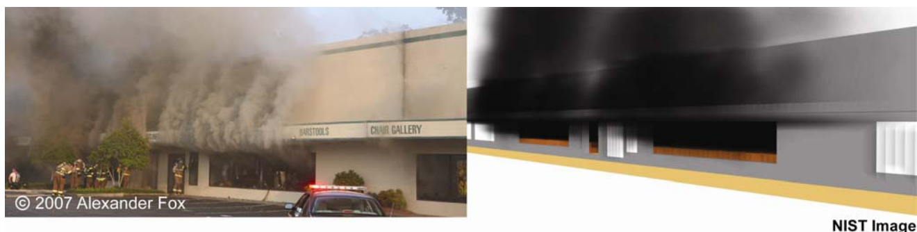
Figure 4-21. Comparison between photo and rendered image from the simulation at 1530 s (7:36:23 p.m.). The view is of the front of the main showroom.
