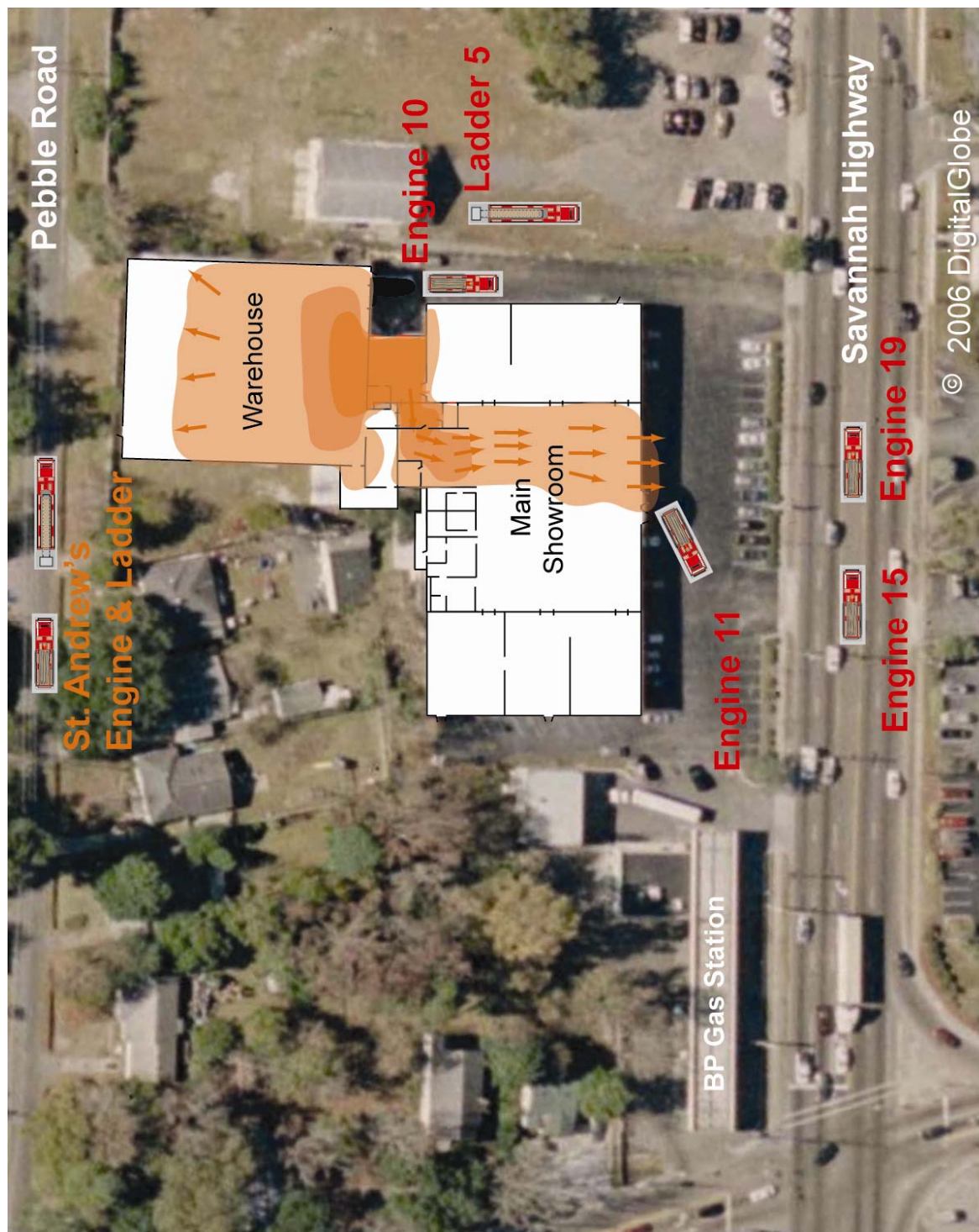
Figure 2-8. Fire spread rapidly from rear of main showroom to the front of the main showroom. Fire continued to spread towards rear of warehouse. This occurred by about 7:36 p.m. Background image used with permission of DigitalGlobe. Enhancements by NIST.
