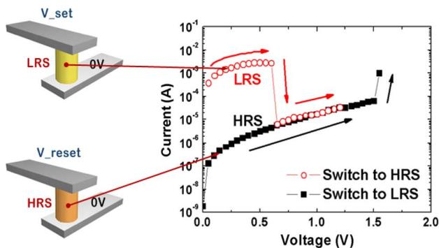
**Fig. 4.** Schematic diagram and typical switching characteristics of an inflexible NiO unipolar resistive switching device. Ramps for switching to the LRS and back to the HRS are shown. Reprinted with permission from [29] © 2008, Wiley-VCH Verlag GmbH & Co.
