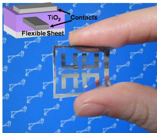
**Fig. 1.** Top view of four flexible memristors and a side view of the flexible memristor structure. Reprinted with permission from [18].
