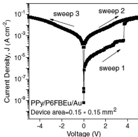
**Fig. 7. Switching characteristics of a flexible polymer WORM device.** Reprinted with permission from [5] © 2007, Elsevier.
