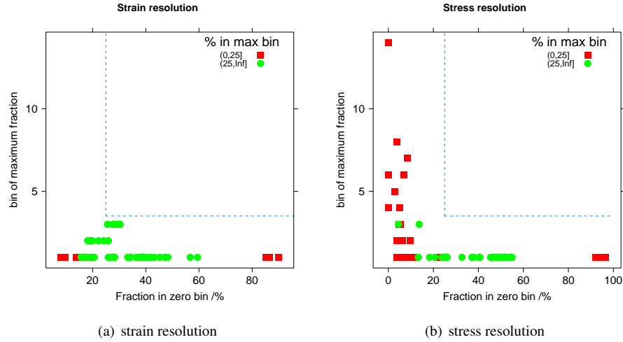
Figure 14: (a) Strain and (b) stress data resolution. Dashed lines enclose the region of insufficient resolution. Symbols denote the fraction of points in the bin of maximum fraction.
