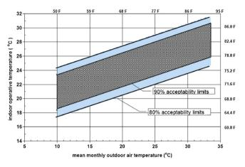
**Fig. 2.** Acceptable operative temperature ranges for naturally conditioned spaces (Copyright 2004 ASHRAE. Reprinted from ASHRAE Standard 55–2004 [4]).
