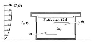
Fig. 1. Single-zone model of a building.
