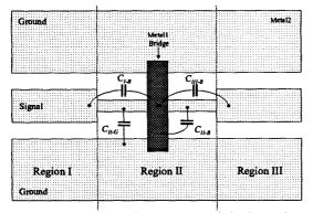
**Figure 3:** Ground equalizers are modeled with a shunt lumped capacitance  $C_{ge}$ . Although, this quasi-static capacitance is dominated by  $C_{II-B}$  in many cases, if *l* is <2w then the contributions from  $C_{I-B}$  and  $C_{III-B}$  are substantial. If I>3w, on the other hand, then  $C_{II-G}$  should be considered as well.
