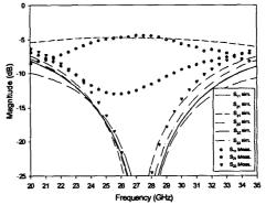
Figure 6: Simulated response of micromachined BLC with measured on-chip 50  $\Omega$  termination.
