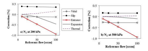
Figure 7. Corrections applied for the circular segment LFM for nitrogen at a)  $P_2 \approx 200$  kPa and b)  $P_2 \approx 500$  kPa.
