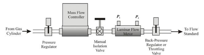
Figure 1. Schematic of the test arrangement to calibrate the laminar flow meters against the PVTt and RoR flow standards.
