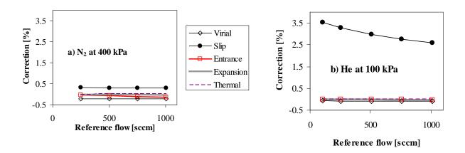
Figure 5. Corrections applied for the annular LFM for a) nitrogen at  $P_2 \approx 400$  kPa and b) helium at  $P_2 \approx 100$  kPa.
