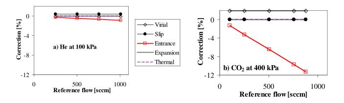
Figure 3. Corrections applied for the circular LFM for a) helium at  $P_2 \approx 100$  kPa and b) carbon dioxide at  $P_2 \approx 400$  kPa.
