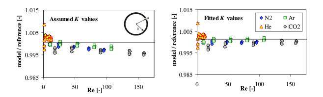
Figure 4. Flow ratio versus Reynolds number for the annular LFM.
