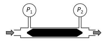
Figure 9. Longitudinal cross section of the annular LFM. The gas flowed through the small gap between concentric cylinders. The tapered end of the inner cylinder reduced turbulence in the gas exiting the gap. The inner cylinder used in the circular segment LFM cylinder had a similar taper.
