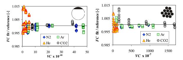
Figure 8. Flow ratios when commonly used flow coefficient versus viscosity coefficient plots are applied to two of the three LFMs. Residuals are as much as 4 times worse than the LFM model.
