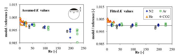
Figure 6. Flow ratio versus Reynolds number for the circular segment LFM.
