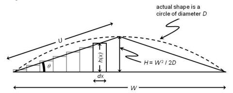
Figure 10. The flow through the very obtuse triangle is approximately the sum of a set of flows through parallel plates.
