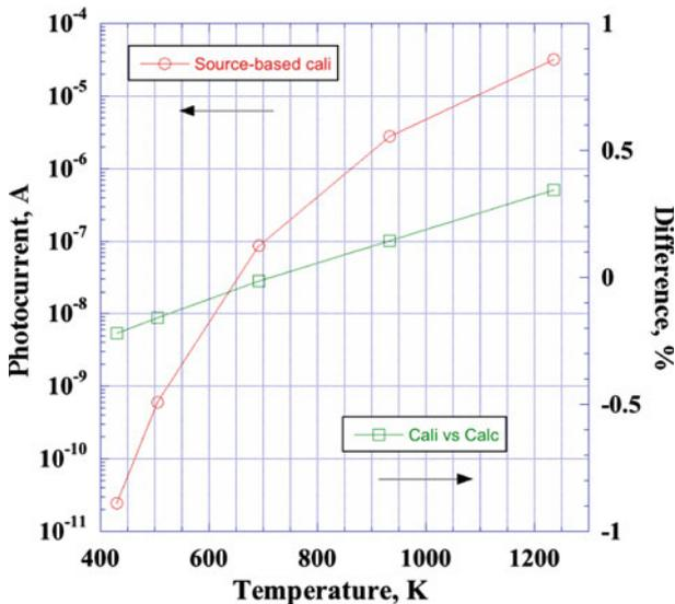
**Fig. 7** NIRT-measured signals versus temperature; agreement of the calculated NIRT signals (from the absolute spectral radiance responsivity) to the measured NIRT signals of five fixed point blackbodies
