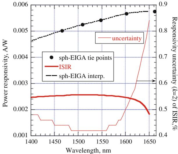
**Fig. 2** Spectral power responsivity of the ISIR based on the interpolated SIRCUS tie points of a sphere-input extended-InGaAs (sph-EIGA) detector
