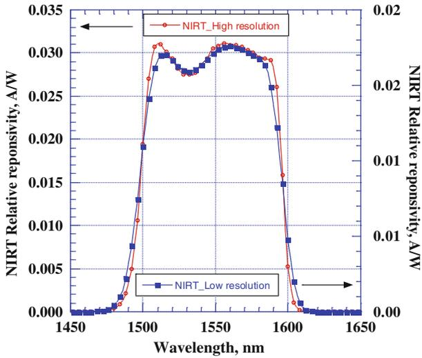
**Fig. 6** Relative spectral responsivity of the NIRT measured with a small and a large slit-width using two different  $Y$ -scales for the two measurements
