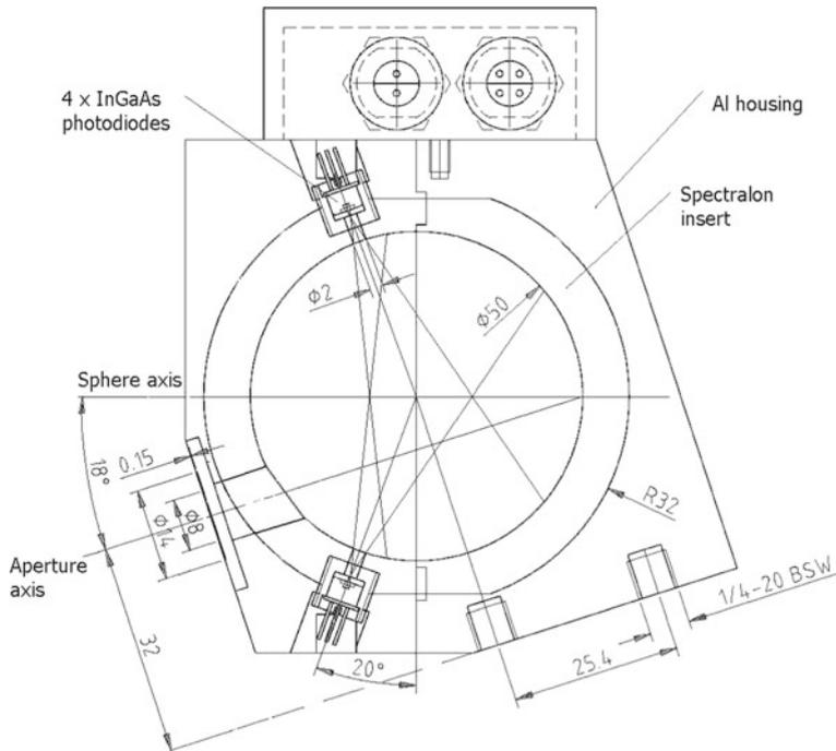
**Fig. 1** Cross section of the sphere-InGaAs (ISIR) reference radiometer
