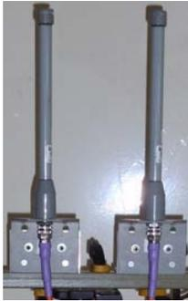
**Figure 4:** Antennas used at receive and transmit locations. Omnidirectional antennas were mounted on a fiberglass rod. The spacing between them was variable.
