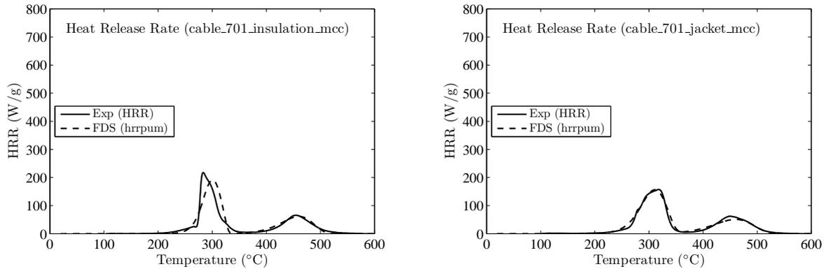
Figure 1: Results of a micro-calorimetry analysis of a sample of cable insulation (left) and jacket material (right).
