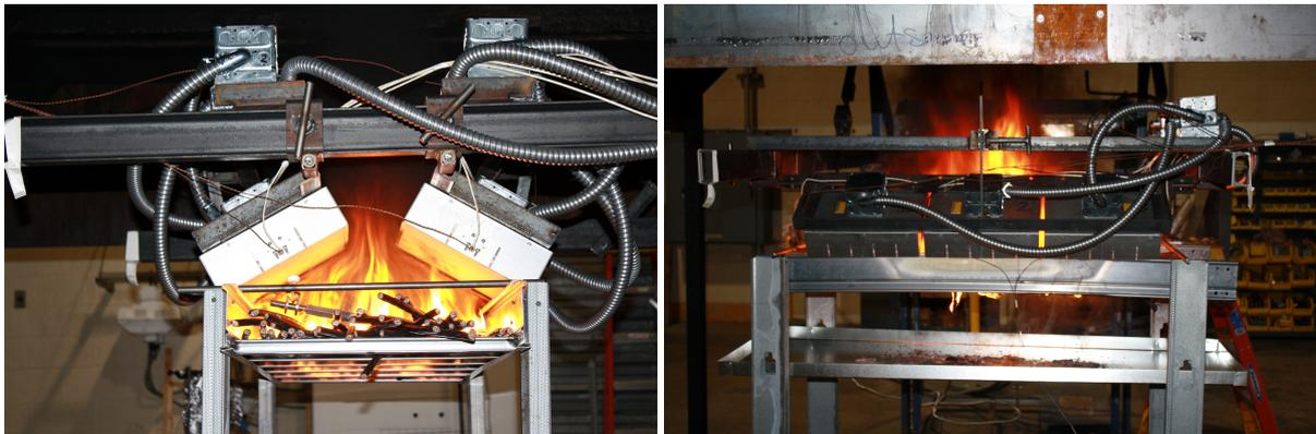
Figure 2: End and side views of the Radiant Panel Apparatus.
