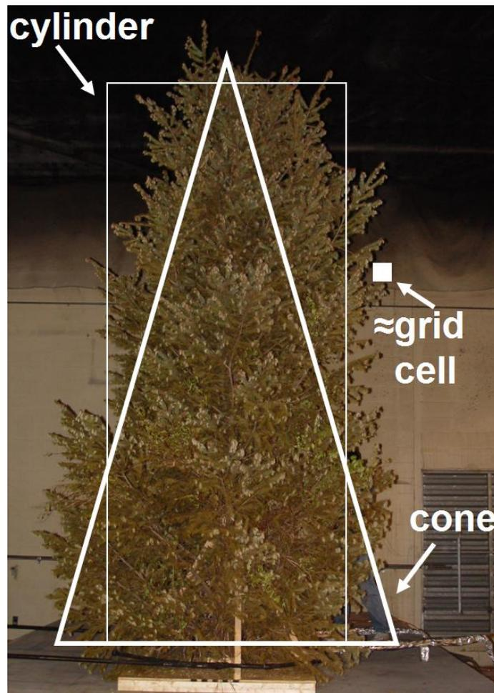
Figure 5: Photograph of 5 m tall Douglas fir with the outlines of the cross sections of both a conical and a cylindrical volume approximation to the tree crown. For simplicity the model approximates the tree as a cone or a cylinder. The approximate size of a grid cell (10 cm) is also shown.
