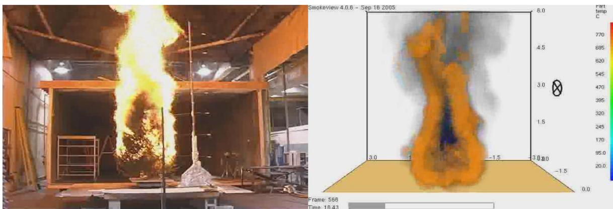
Figure 6: Experiment and simulation of a burning fir tree.
