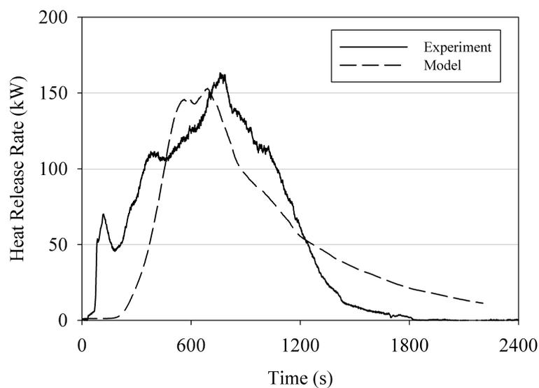
Figure 4: Comparison of predicted and measured heat release rate of burning cables in the Radiant Panel Apparatus.
