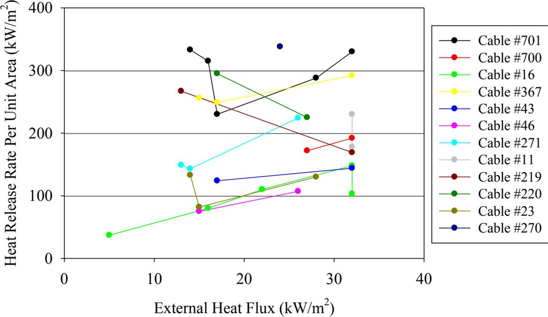
**FIGURE 8. Summary of the radiant panel heat release rates.**
