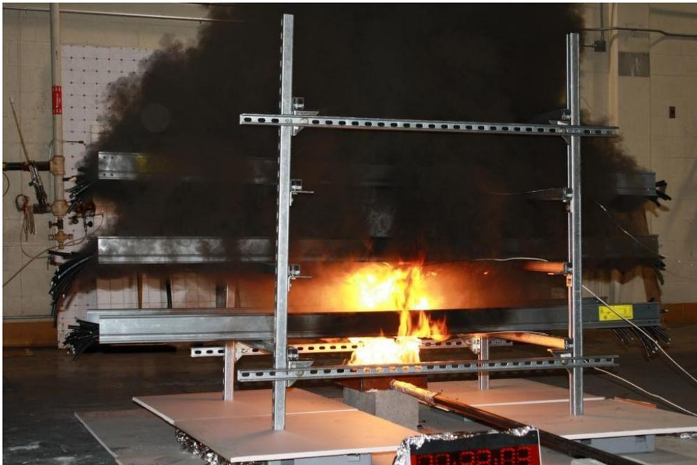
**FIGURE 4. Multiple Tray (MT) cable test apparatus.**
