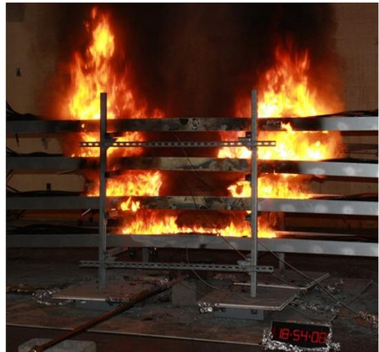
**FIGURE 10. Results of a multiple tray test involving a thermoplastic cable. The vertical lines indicate when each tray became fully involved in the fire. Tray 1 refers to the lowest tray. Note that the involvement of Tray 1 coincided with the extinguishment of the burner.**
